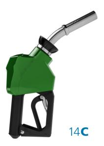
**14C Diesel Capture Technology** – Free-draining spout with patented and patent-pending diesel-capture technology. A specially designed chamber inside the nozzle safely captures diesel fuel draining inside and outside the spout when the nozzle is returned to the cradle. The unique diesel-capture chamber allows the nozzle venturi to evacuate captured diesel fuel from the chamber and reintroduce it into the fuel stream. It's safe, durable and easy to use. The 14C is cULus Listed.
