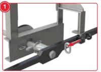
Handle detached, disengaged, and locked in the closed position – bottom outlet ball valve and commodity are safe and secure for transport
