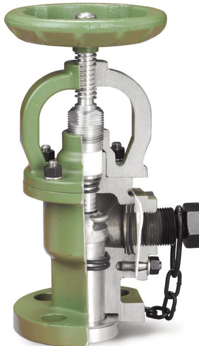
the packing rings. This live loading compensates for packing wear and thermal expansion and contraction of the packing when flashing in the valve occurs. The valves also incorporate secondary adjustable stem packing, providing improved stem sealing and The A-713 is also equipped with a replaceable outlet port that can be easily replaced without removing the valve from the tank car or truck.
