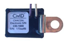
The Civacon CivID Model CID-1000 Electronic Serial Number provides a unique electronic serial number to loading rack monitors equipped to automatically read this industry standard format number. This electronic serial number is used by the terminal automation system to electronically identify the cargo tank. The CivID Model CID-1000 mounts inside the cargo tank's overfill prevention socket housing and simply wires to pins #9 & #10 inside the socket.
