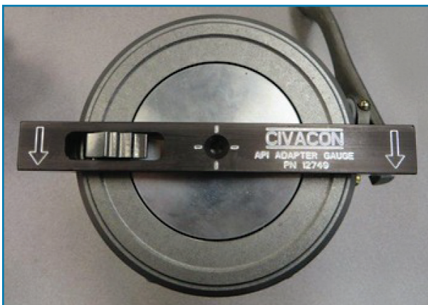
API adaptor shown with API Adaptor Wear Inspection Gauge attached
