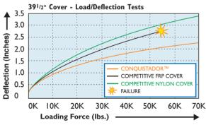
The Conquistador™ Duratuff's unique structural fiberglass construction provides load strength and durability performance that are unmatched.
