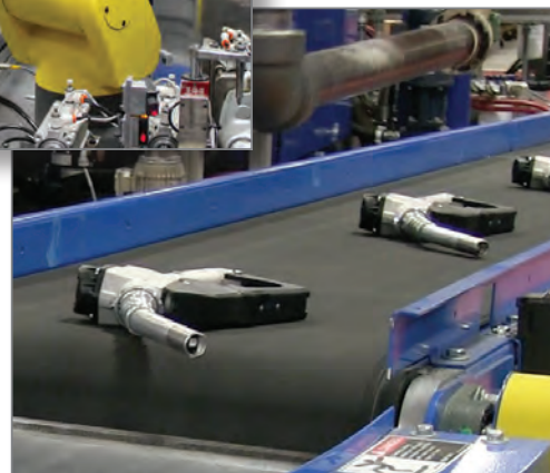
OPW's fully robotic line with automated nozzle assembly and testing.
