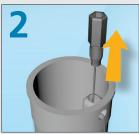
LIFT FLOAT WITH CABLE TO SIMULATE FILL
