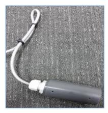
Step #3: Remove the protective end cap from the sensor to access the float.
