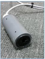
Step #4: Remove the cotter key that holds the float in place and remove the float gently.
