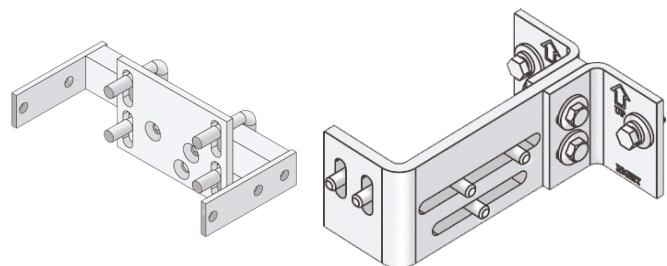
**IMPORTANT:** Stabilizer bars must be tightened down securely to the side strut after the dispenser has been mounted.
