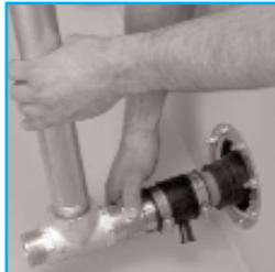
**Step 3:** Install stabilizer bars to dispenser sump riser frame. Attach shear valves to stabilizer bars. Install anchor bolts to the dispenser sump frame.
