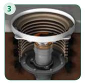
Replace Bellows, Reinstall Upper and Lower Rings
