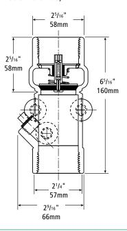
Warning: The valve body must be rigidly anchored to a structural member within the island to ensure breakage at the shear groove in the event of severe impact. The shear groove must be at the same level or a maximum of 1/2" above or below the top of the pedestal island. Failure to provide rigid mounting or install the shear groove at the proper level may result in a failure of the valve to close or shear, resulting in an excessive loss of product and a hazardous condition.
