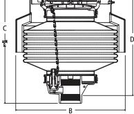
NOTE: "D" dimension is height from riser pipe to finish grade (+1" for slope)
