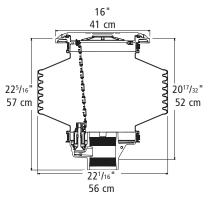
\*Subtract 2" from height dimension for Cast Iron Base Models.
