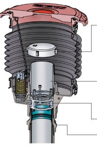
OPW 1-2100, 5-Gallon 16" 41 cm 16<sup>17</sup>/32" 42 cm Height 18<sup>11</sup>/32 from Riser 47 cm Pipe To Finished Grade (+1" for slope) 14<sup>1</sup>/16 36 cm
