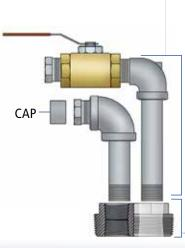
PDT-411 FlexWorks Double-Tapped Tank Bung Fitting, 4" (10 cm) MNPT w/Dual 1" (3 cm) FNPT Taps - Used in 4" (10 cm) Tank Bung to accommodate FOP Supply and Return Lines
