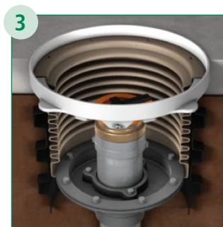
Replace Bellows, Reinstall Upper and Lower Rings
