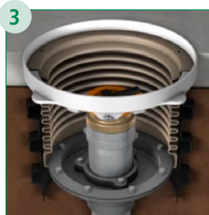
3 Replace Bellows, Reinstall Upper and Lower Rings
