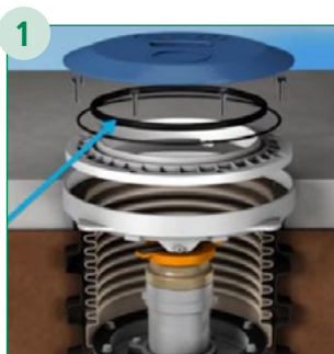
1 Remove Upper Bolts and Ring
