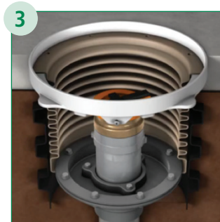
Replace Bellows, Reinstall Upper and Lower Rings
