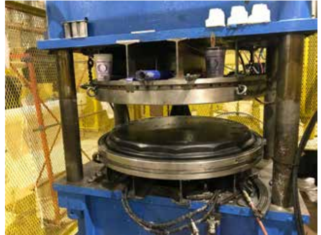
The Resin Transfer Molding (RTM) production process saturates glass fibers with resin to create the fiberglass then uses a hydraulic press to compress the two halves of the part together, resulting in a smooth, leak-free finish.
