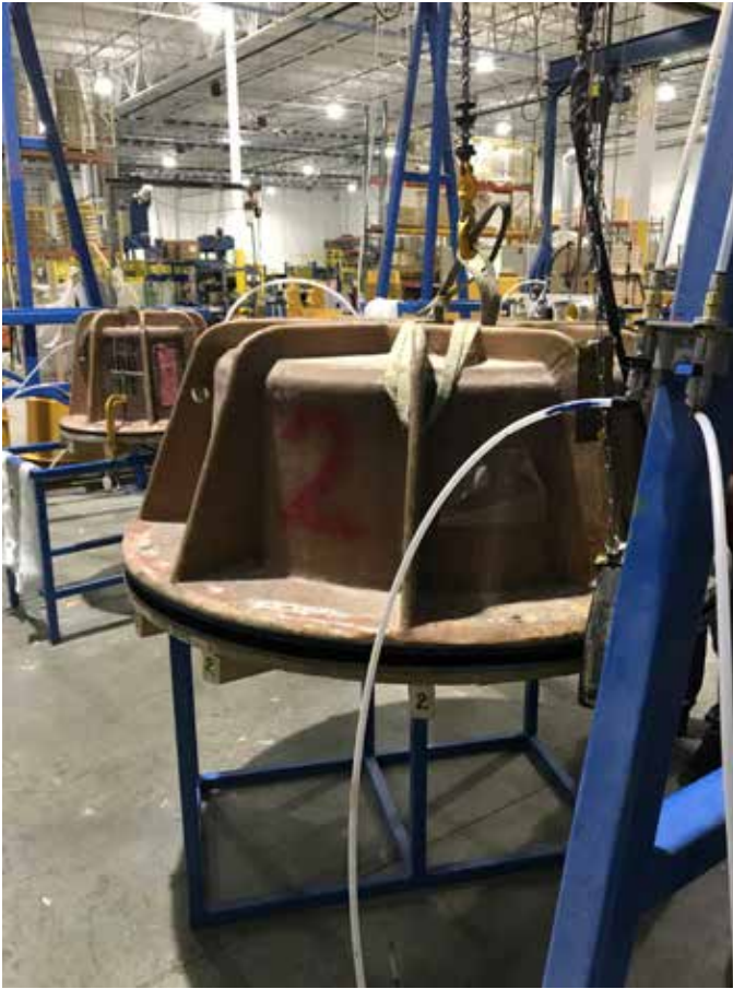
The Vacuum-Assisted Resin Transfer Molding (Vac-RTM) process builds on the benefits of RTM fiberglass manufacturing through the use of a vacuum that helps create incredibly smooth walls that have no porous or weak spots that can compromise performance.
