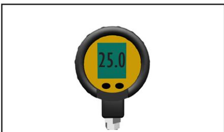
Pressure test the pipe at 25 bar (363 psi) or according to local regulations, but max 40 bar (580 psi).
