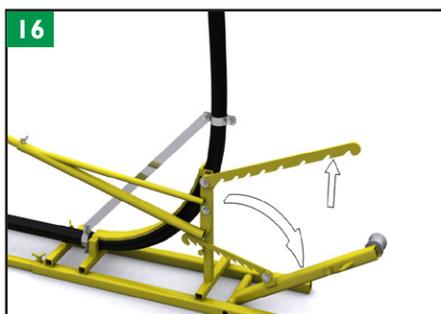
Press the handle slightly and release the locking mechanism.
