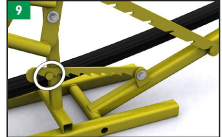
When the locking device clicks into the first notch, release the handle.
