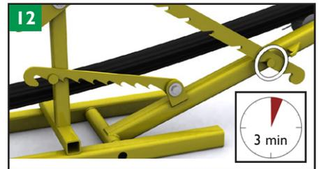
Release the handle and wait for 3 minutes. Repeat the process until the pipe is fully bent. Pause 3 minutes between each notch.
