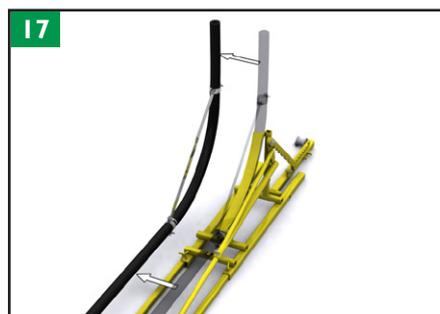
Remove the pipe from the bending tool.
