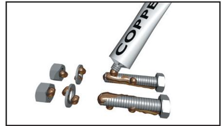
Lubricate stainless steel bolts, washers and nuts with copper paste, ceramic paste or MoS2.
