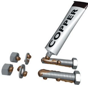
All threads on bolts and nuts must be lubricated with copper paste, ceramic paste or MoS<sub>2</sub>.
