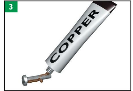
Lubricate the smaller mounting screw using copper paste, ceramic paste or MoS<sub>2</sub>.
