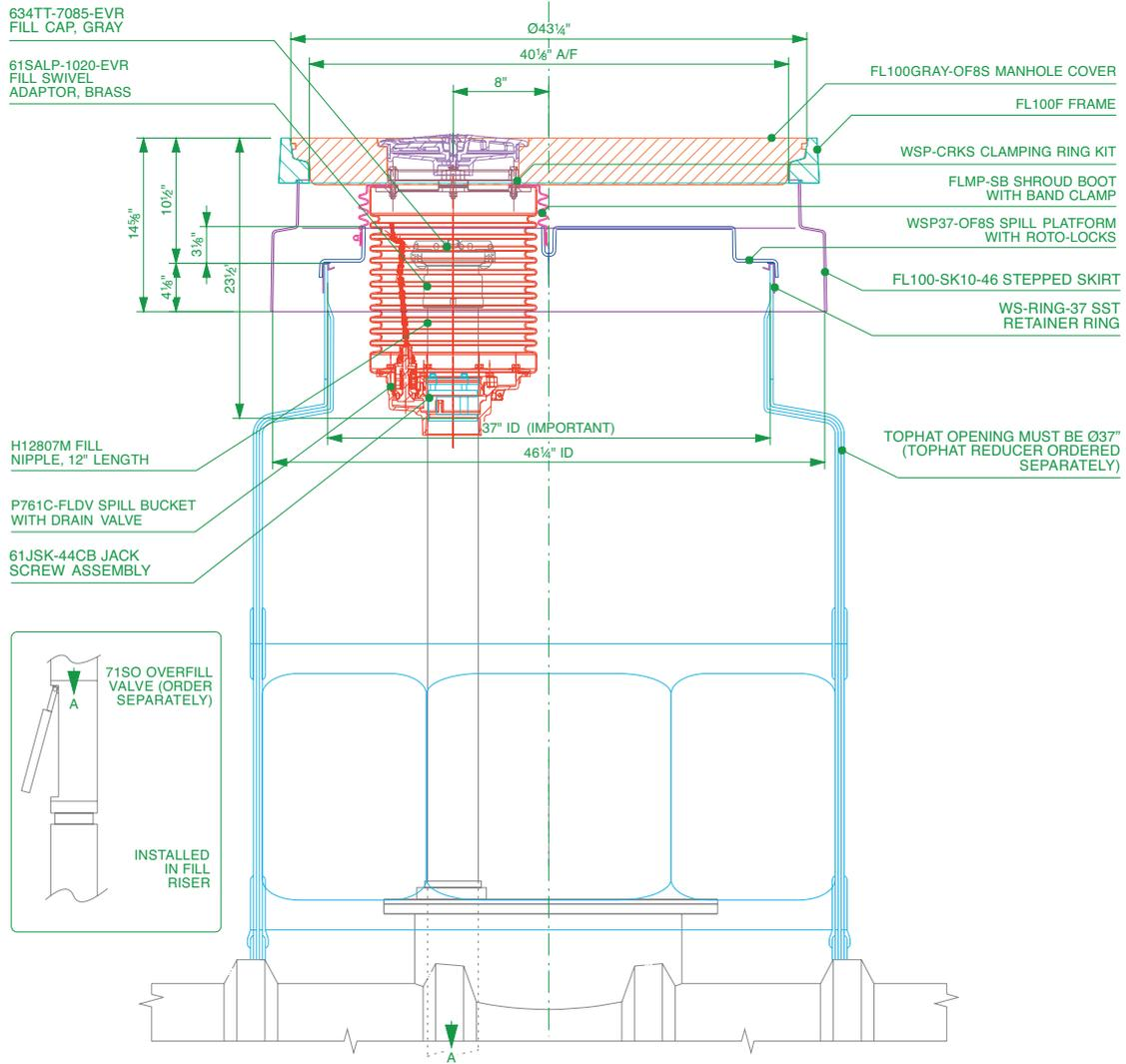
FibreTite multiport kit includes watertight platform for (1) 5-gallon spill bucket, 40" diameter offset cover, port cover, frame and skirt.
