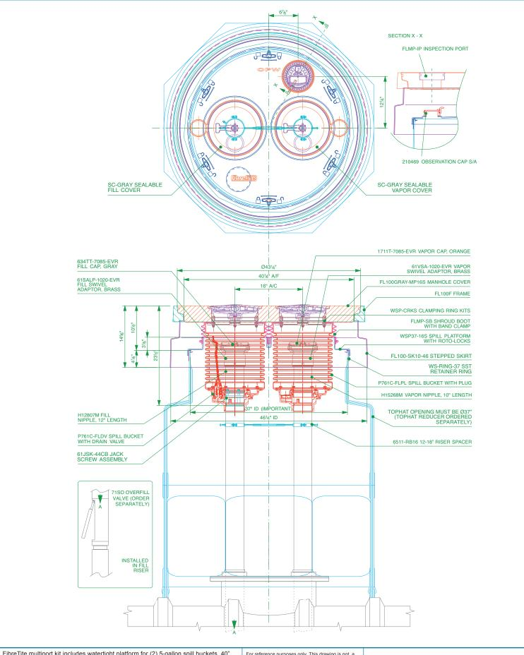
FibreTite multiport kit includes watertight platform for (2) 5-gallon spill buckets, 40" diameter multiport cover, port covers, frame and skirt.
