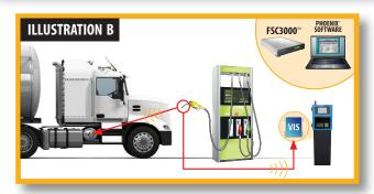
When the RFN locates the Passive Vehicle Tag it transmits back to the VIS, reporting the vehicle's tag number.
