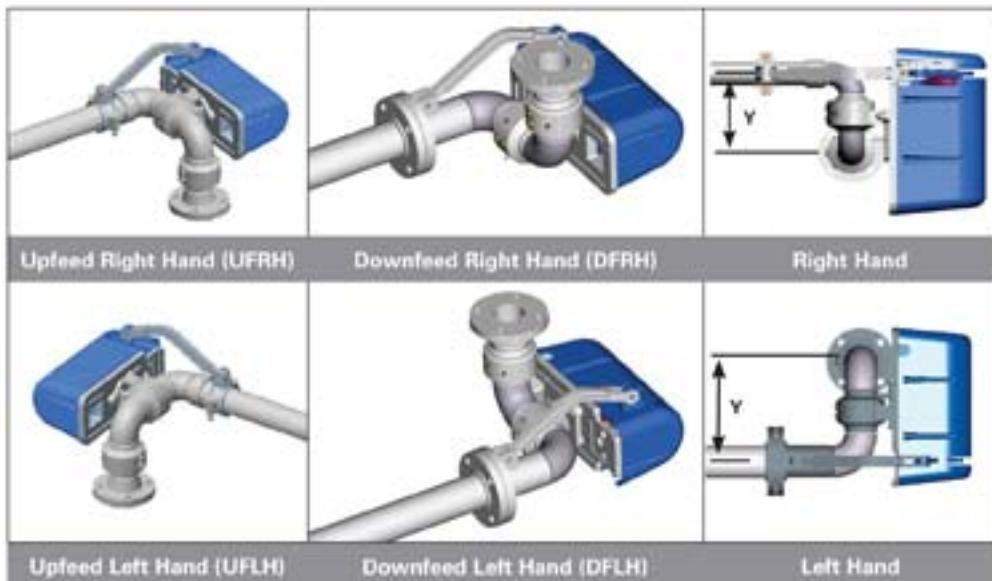
Maximum Y-dimensions: 2" size:  $Y=8\frac{1}{8}$ " (207 mm); 3" size:  $Y=11$ " (280 mm); 4" size:  $Y=12$ " (324 mm); and 6" size:  $Y=18$ " (470 mm).
