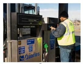
The OPW FSC3000<sup>™</sup> Fuel Site Controller inside the C/OPT<sup>™</sup> Fuel Island Terminal can track and report fueling transactions by driver and/or vehicle.
