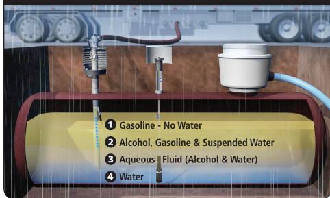
Water can enter tanks in two ways, which are common and difficult to prevent: The spill container during fuel delivery
