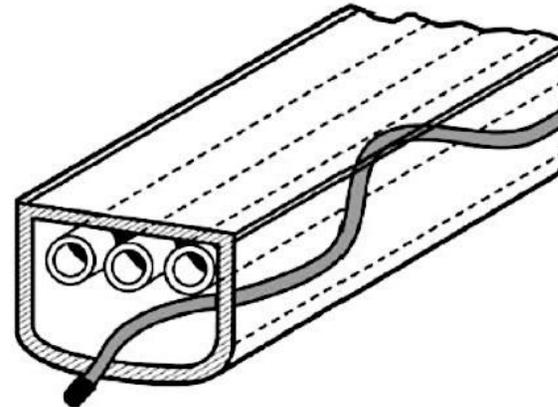
Figure 5-14 Interstitial Sensor Installed in Manway
