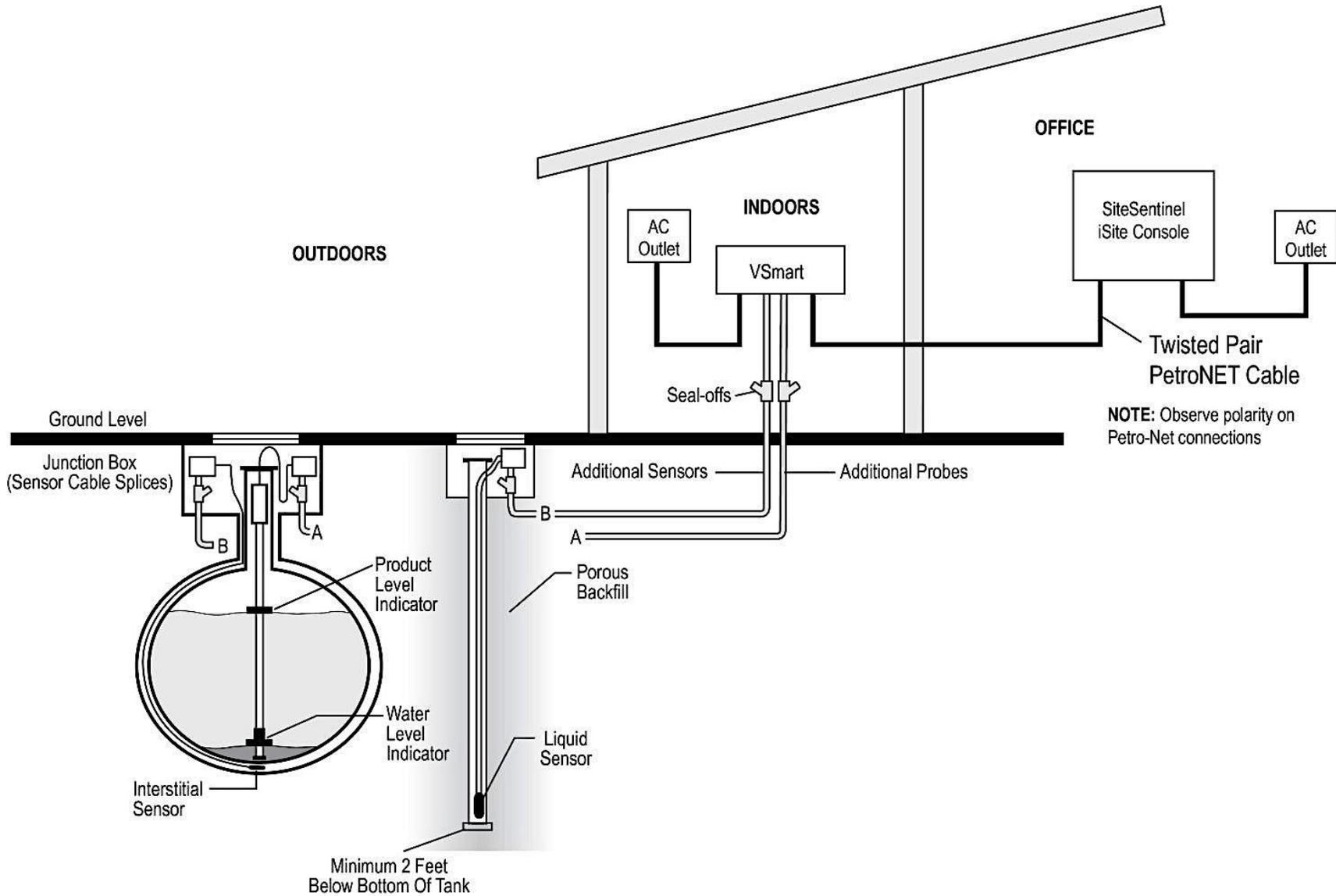
Figure 2-11 Standard Twisted-Pair Petro-Net Installation
