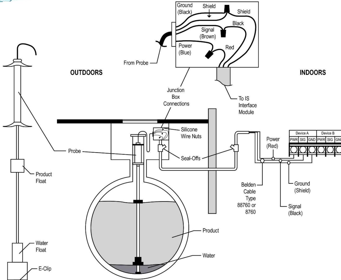
Figure 4-1 924B Probe Installation
