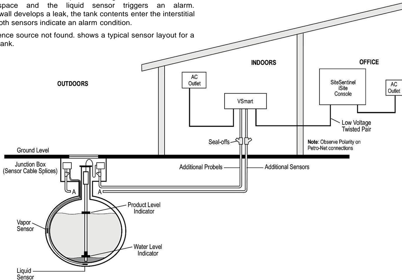
Figure 9-5 No-Well Monitoring, Double-Wall Tank
