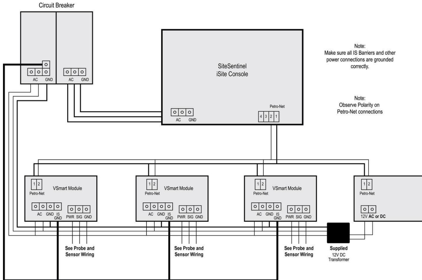
Figure 2-10 Petro-Net and A/C Wiring
