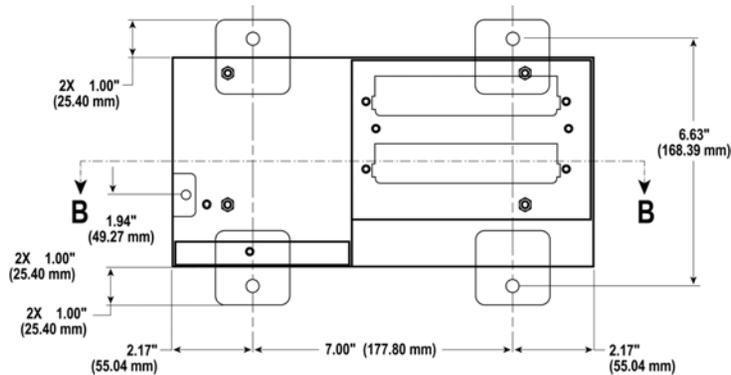
Figure 8-4 VSmart Mounting Dimensions
