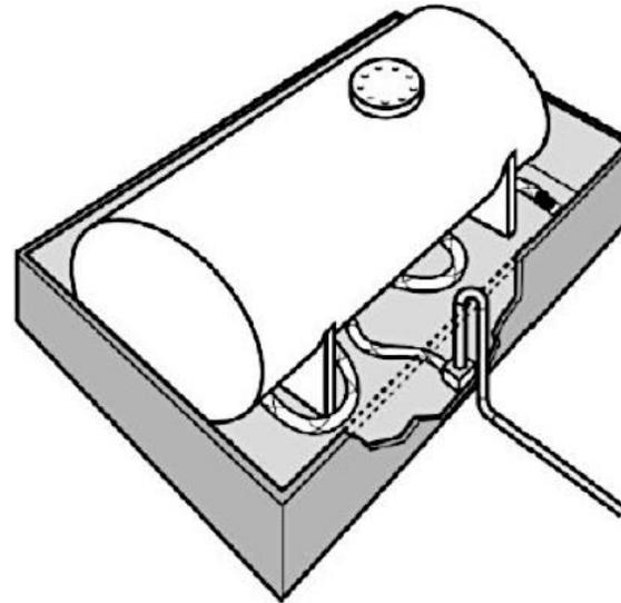
Figure 5-13 Interstitial Sensor in Aboveground Tank
