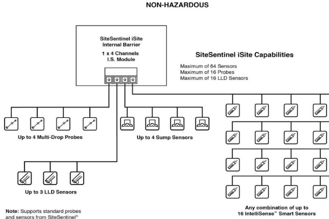
Figure 9-1 Sensor Installation Diagram
