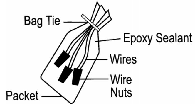
Figure 12-4 Epoxy Sealant Pack
