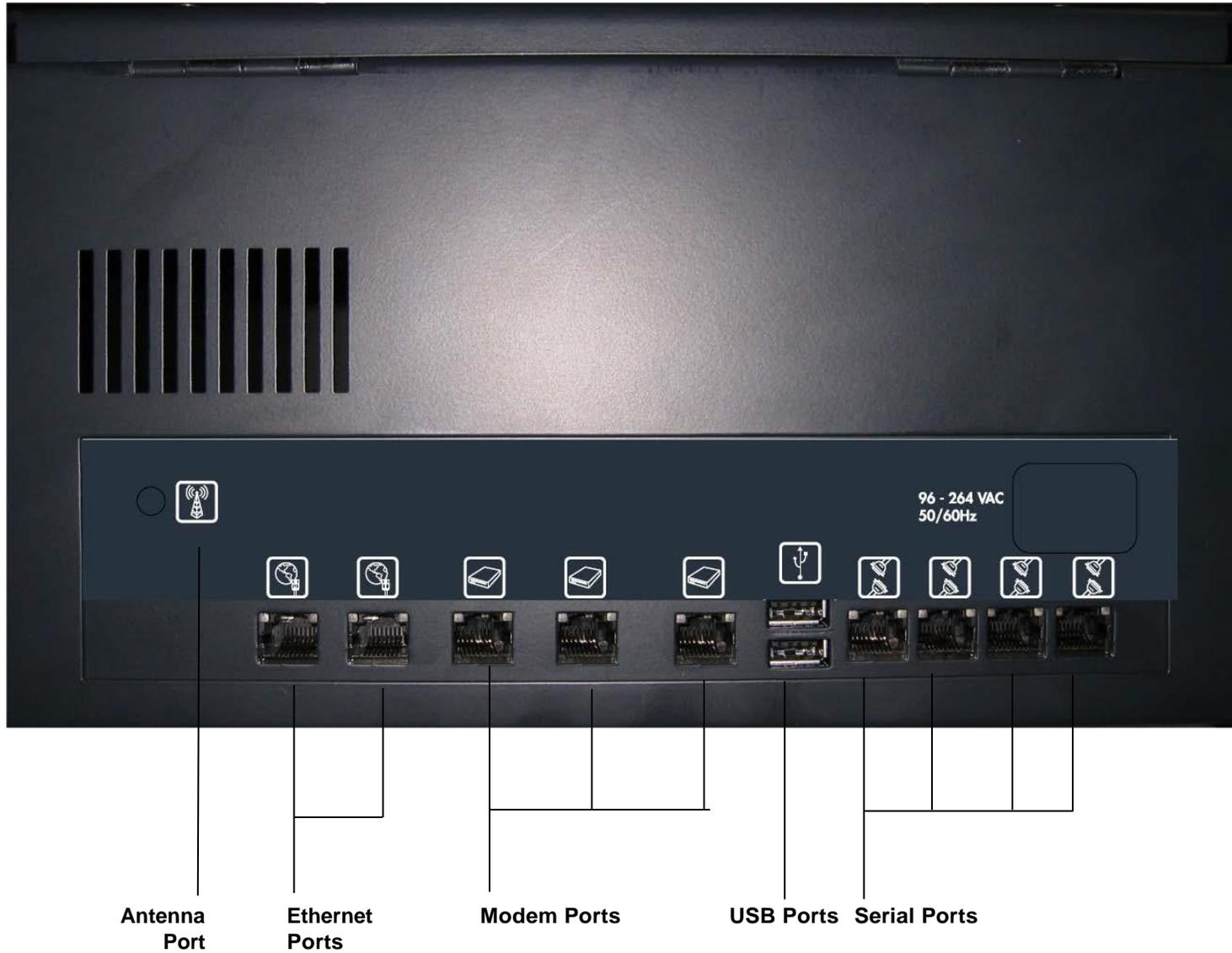
Figure 2-5 Port Connections
