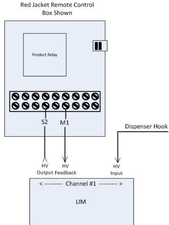
Figure 7-6 Typical Red Jacket Wiring Connections
