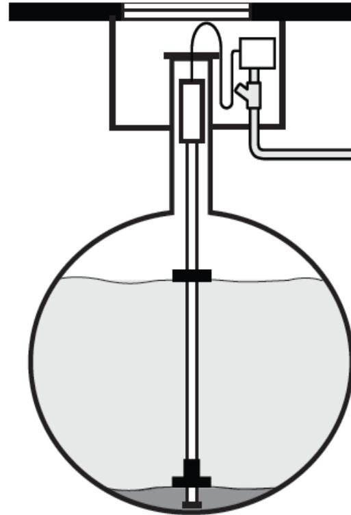
Figure 9-2 Dry Well Monitoring, Single-Wall Tank
