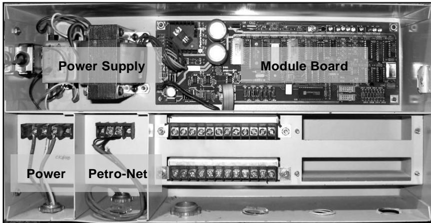
Figure 12-3 SiteSentinel® iSite™ Smart Module Connections
