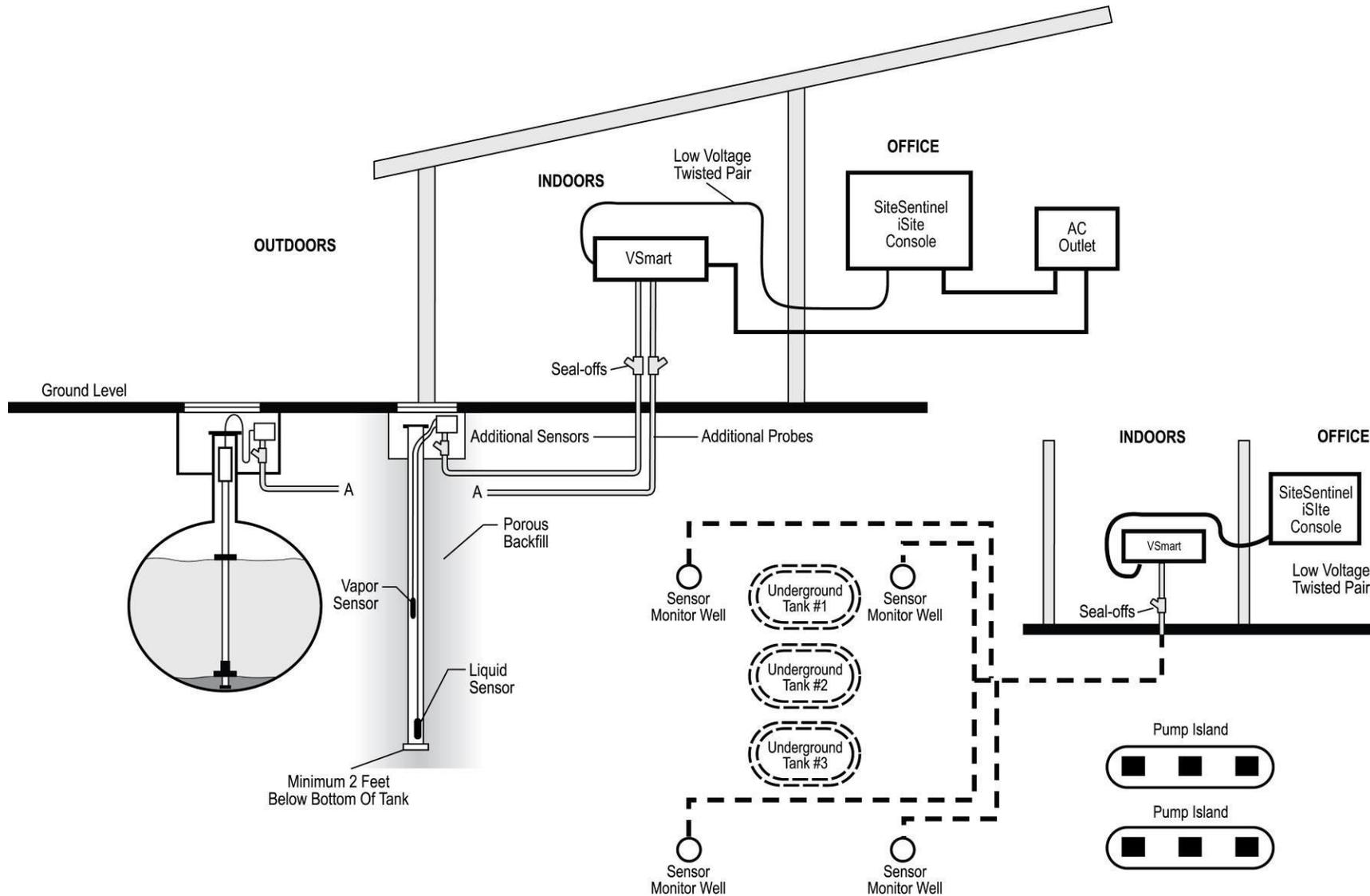
Figure 9-3 Dry-Well Monitoring, Single-Wall Tank
