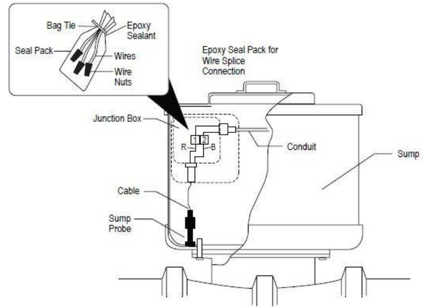
Figure 5-5 Universal Sump Sensor Installation
