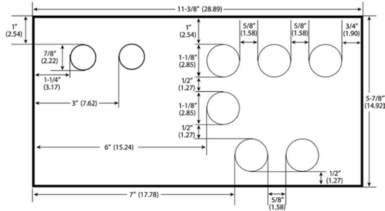
Figure 8-3 VSmart Module Knockouts
