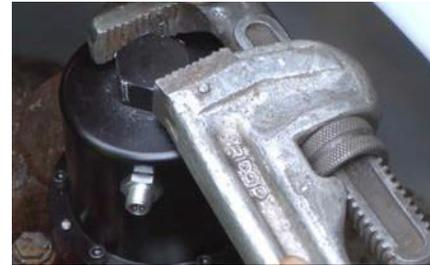
Figure 6-4 Tighten Sensor
