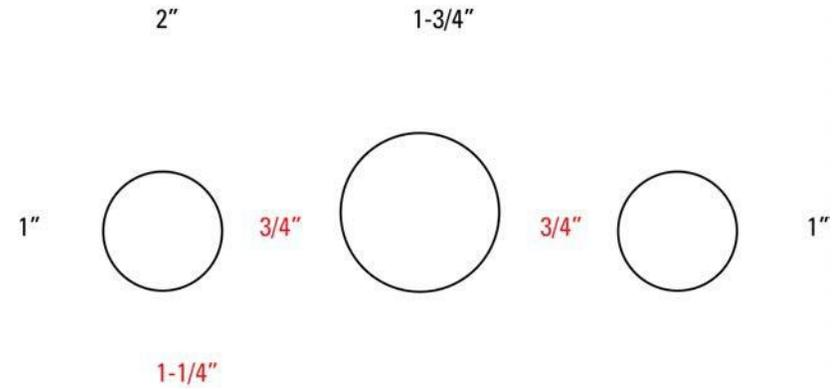
Figure 8-6 I/O Module Knockouts
