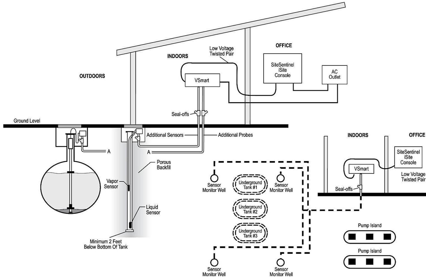
Figure 9-4 Wet-Well Monitoring, Single-Wall Tank
