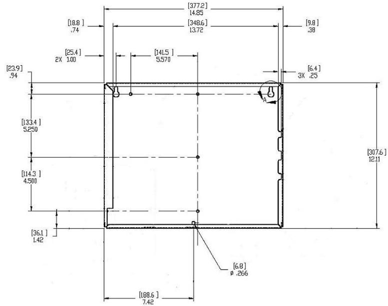
Figure 8-2 Console Mounting Dimensions
