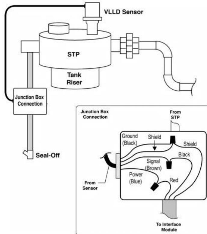
Figure 6-5 VLLD Wiring Connections
