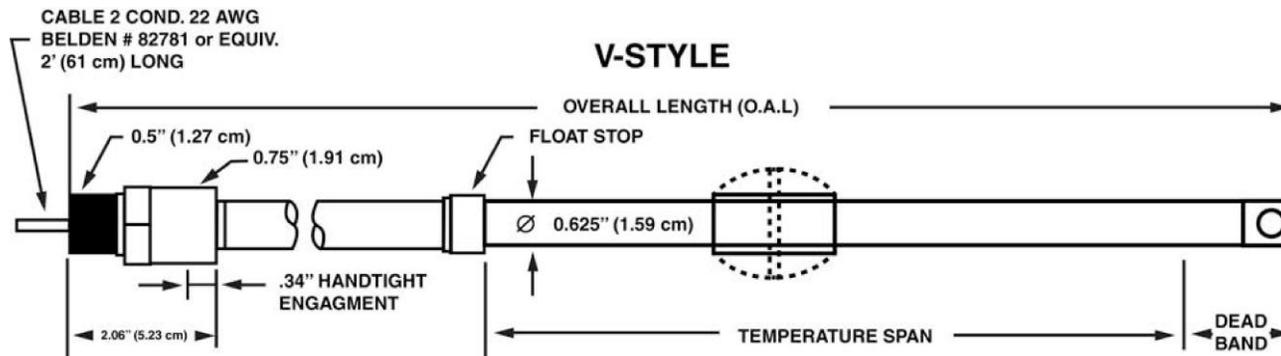
Figure 4-8 Flex Probe Component Diagram
