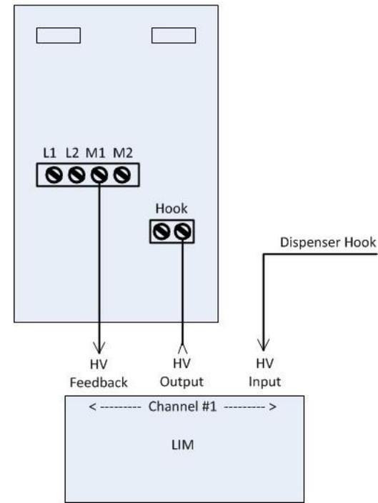
Figure 7-4 Typical FE Petro Wiring Connections
