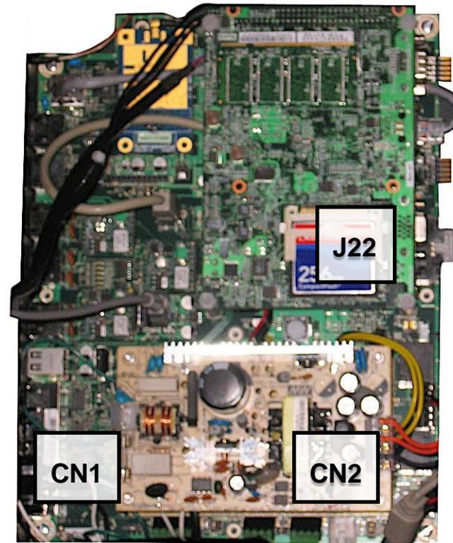
Figure 2-19 Main Board Printer Connections
