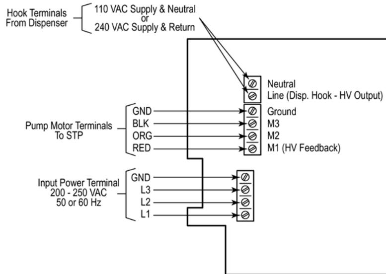
Figure 7-2 Variable Speed Control Wiring for FE Petro
