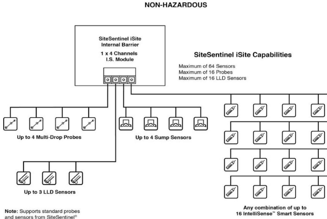
Figure 9-1 Sensor Installation Diagram
