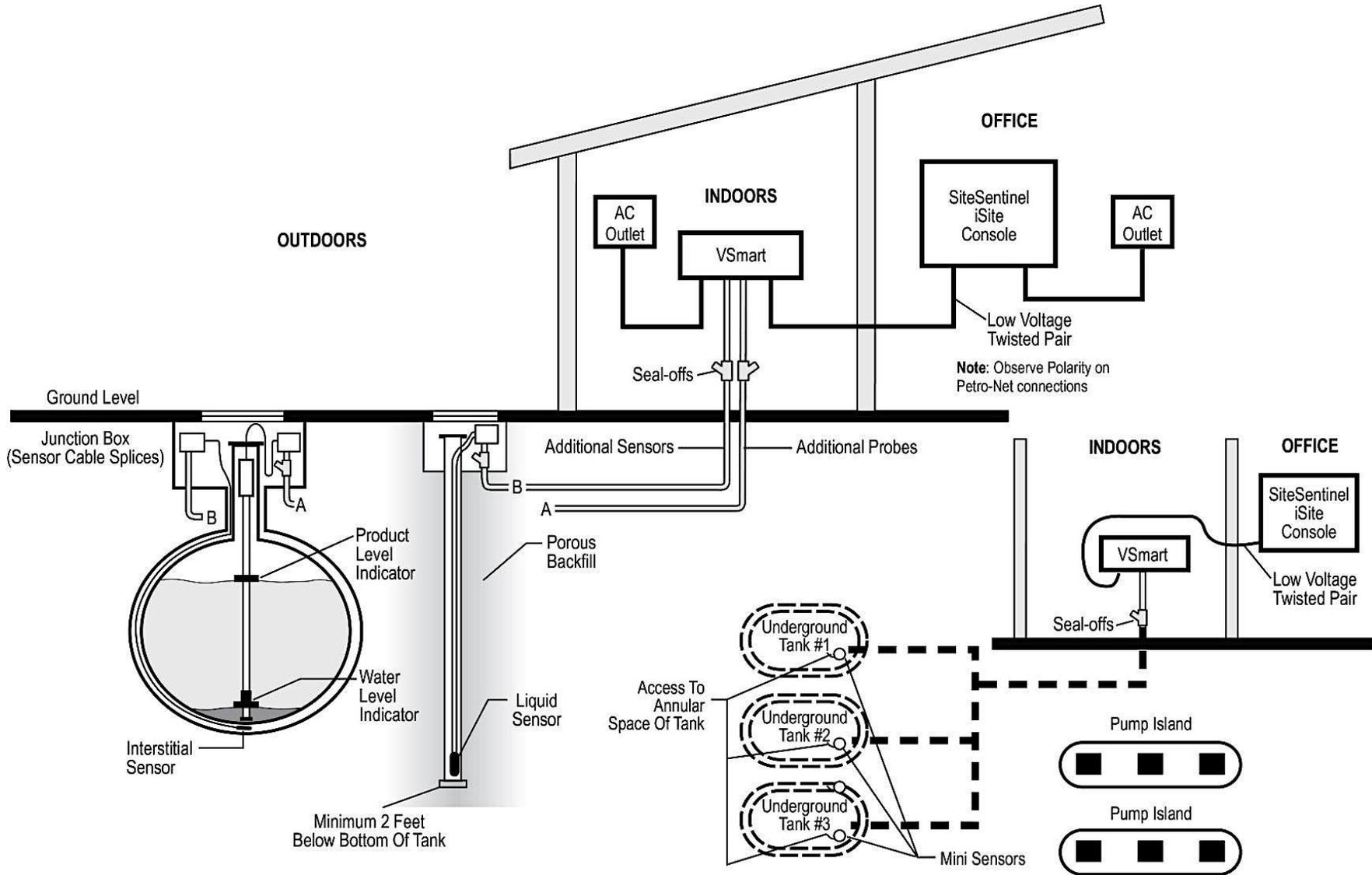
Figure 9-7 Double-Wall Tank with Well Monitoring
