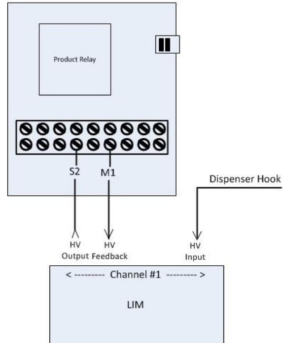
Figure 7-6 Typical Red Jacket Wiring Connections
