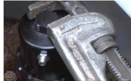
Figure 6-4 Tighten Sensor
