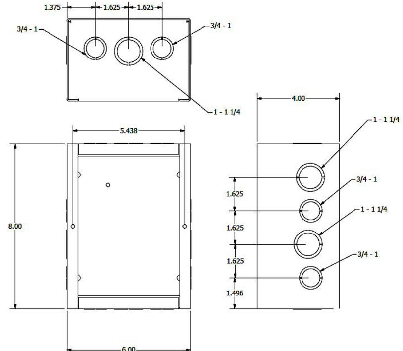
Figure 8-5 LIM Knockouts and Dimensions
