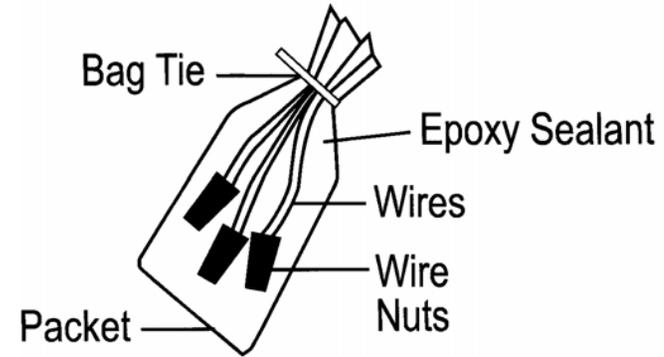
Figure 12-4 Epoxy Sealant Pack
