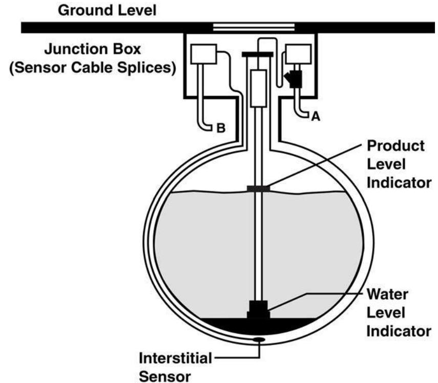
Figure 9-6 Double-Wall Tank with Well Monitoring
