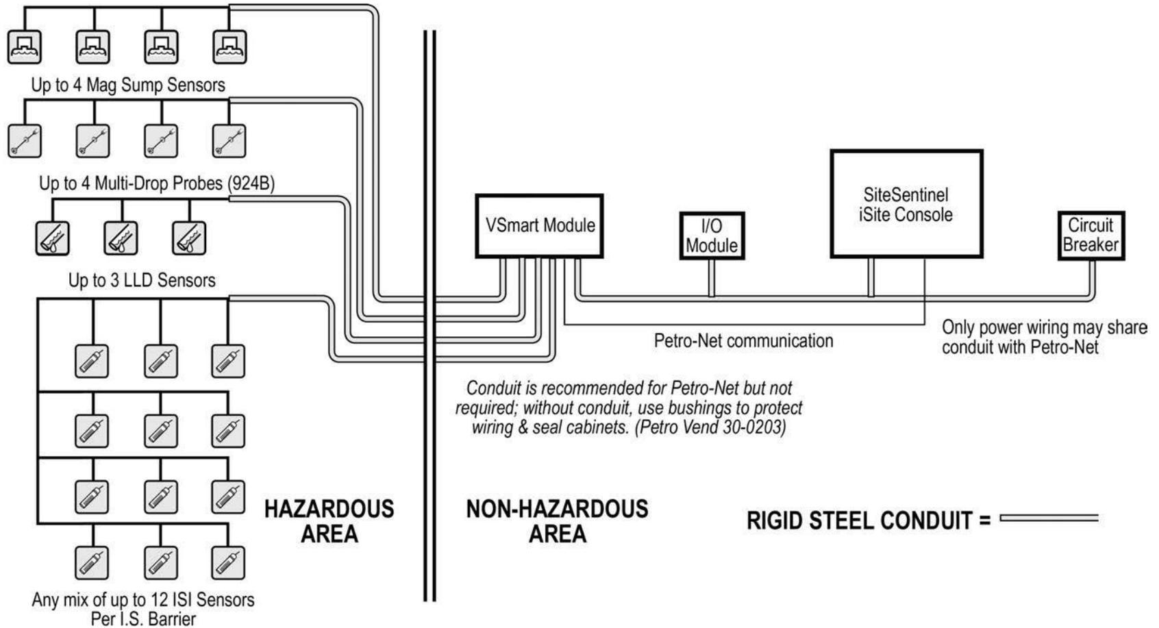
Figure 2-17 Petro-Net Conduit Installation
