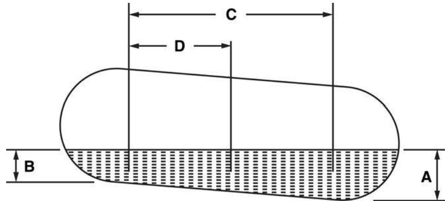
Figure 3-3 Calculating Product Offset in a Tank
