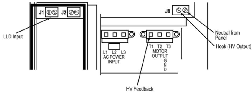
Figure 7-5 Variable Speed Control Wiring for Red Jacket
