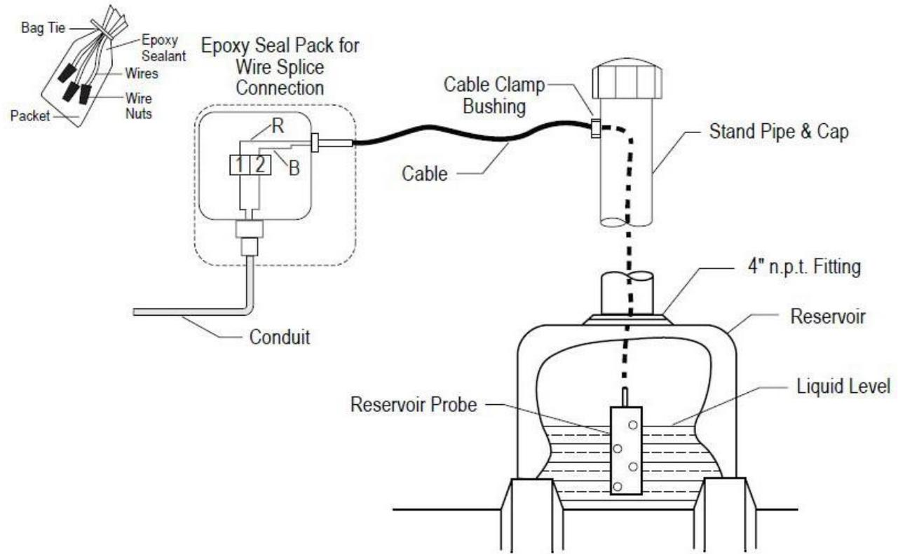
Figure 5-19 Reservoir Sensor Installation
