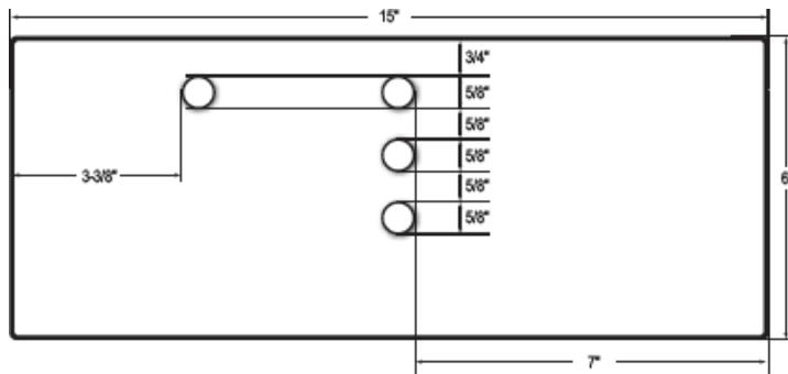
Figure 8-1 Console Knockouts
