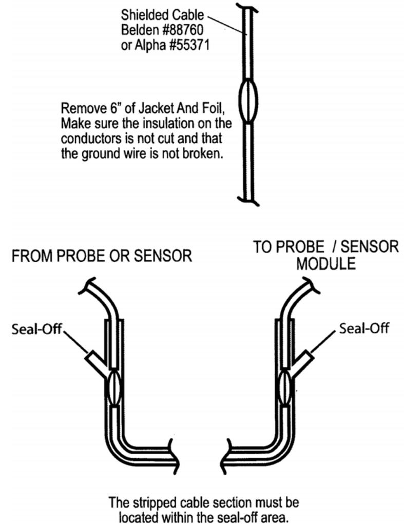
Figure 10-1 Probe-Cable Seal-Offs
