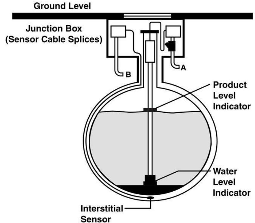
Figure 9-6 Double-Wall Tank with Well Monitoring
