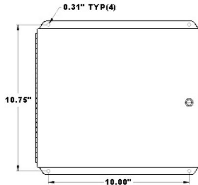
Figure 13-2 ACR/RIM Interface Mounting Enclosure
