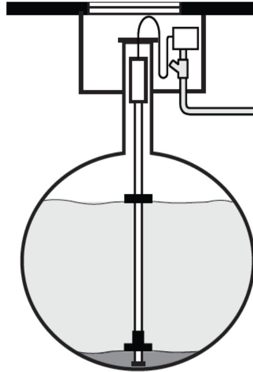
Figure 9-2 Dry Well Monitoring, Single-Wall Tank
