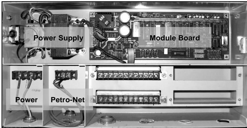
Figure 12-3 SiteSentinel® iSite™ Smart Module Connections
