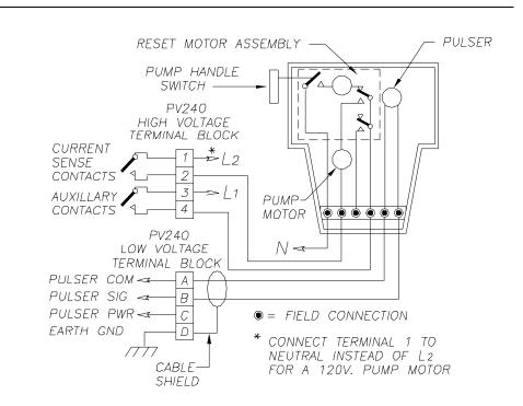
Figure 7: Typical Pump Control Wiring - Self-Contained/Power Reset
