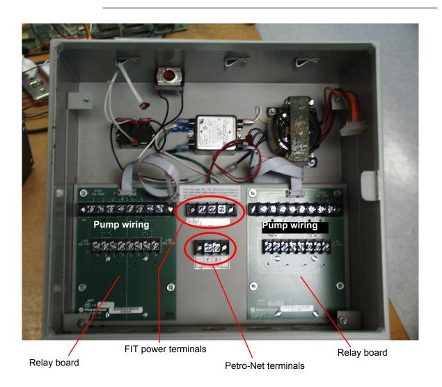
Figure 4: FIT Terminals & Relay Boards
