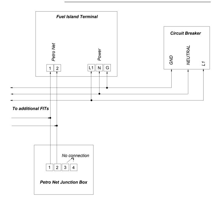
Figure 5: FIT Wiring Overview
