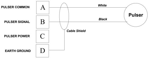
Figure 9: Pulser Wiring -- Veeder-Root 1871
