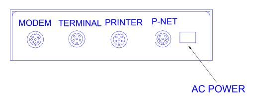
Figure 13: K800 Fuel Site Controller Rear Panel
