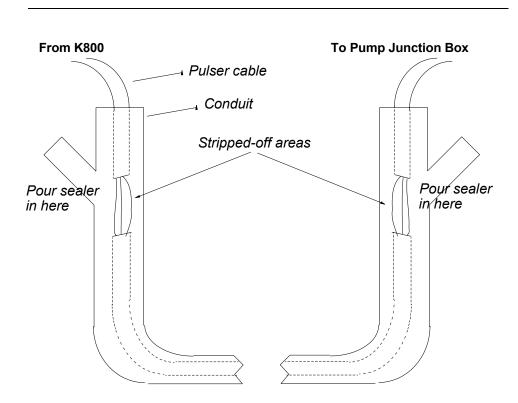
Figure 11: Pulser Seal-Off Concept
