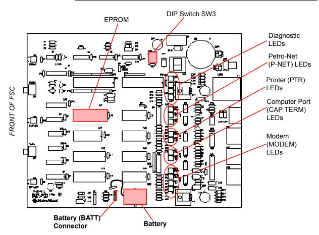
Figure 16: K800 Fuel Site Controller Board
