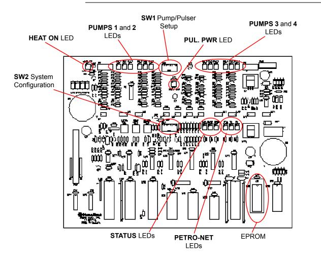
Figure 14: K800 Fuel Island Terminal PC Board
