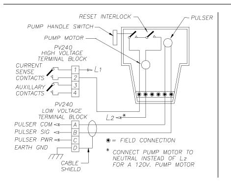
Figure 6: Typical Pump Control Wiring -- Self-Contained
