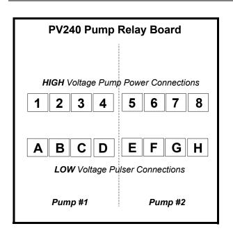
Figure 12: Pump Relay Board Wiring
