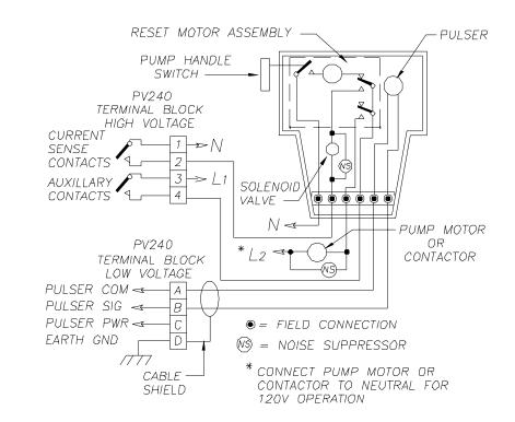
Figure 8: Typical Dispenser Control Wiring
