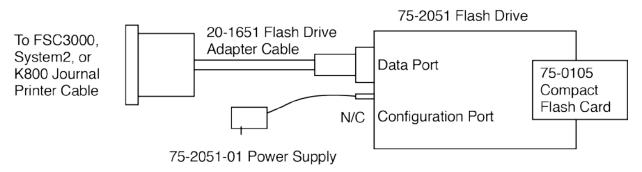
Figure 1-2 Data Recorder Connection Diagram
