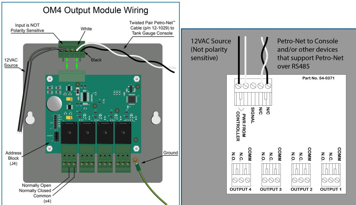
OM4 Wiring Connections and Wiring Instruction Label 54-0371
