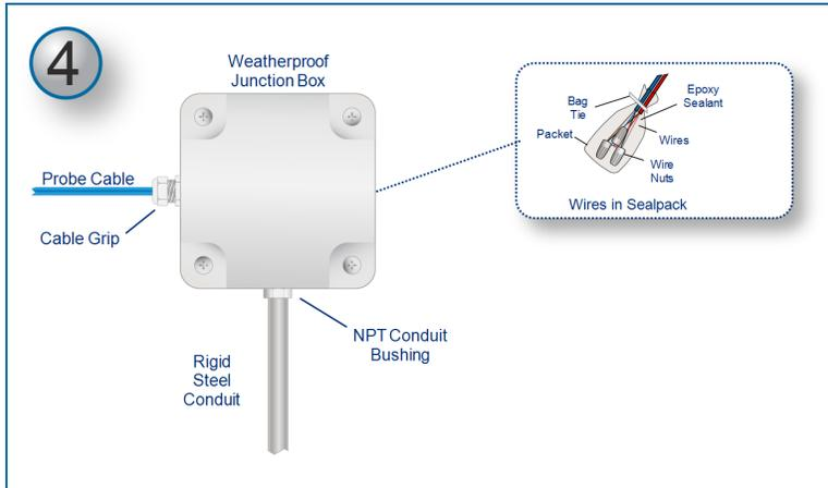
4. Tank-Probe or Smart Sensor wires that use a prepared Belden or Alpha cable must go through NPT bushings into a weatherproof junction box. Bushings must be used in all junction boxes.
