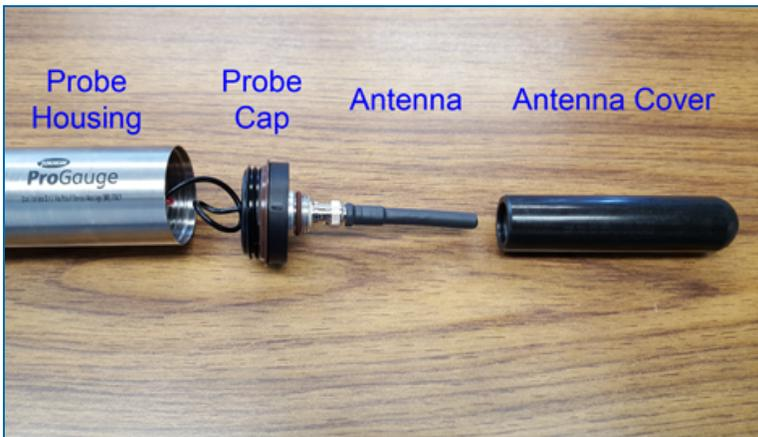
To get access to the probe's inner components (battery housing, probe board with jumper block and DIP-Switches), turn the cap counter-clockwise and carefully remove it from the housing.
