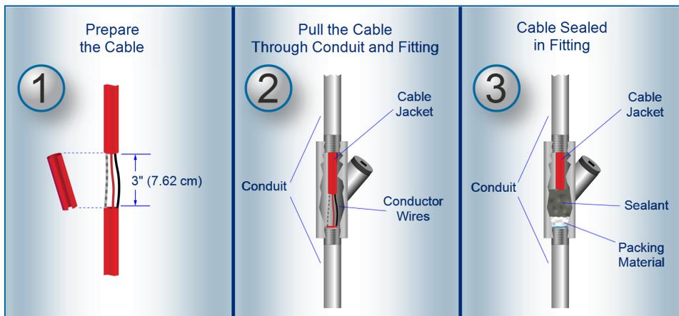
1. Prepare the Cable: Remove a sufficient length of the cable *jacket* so that the *conductor* wires can extend into the conduit seal fitting (approximately 3 inches [7.62 cm]).
