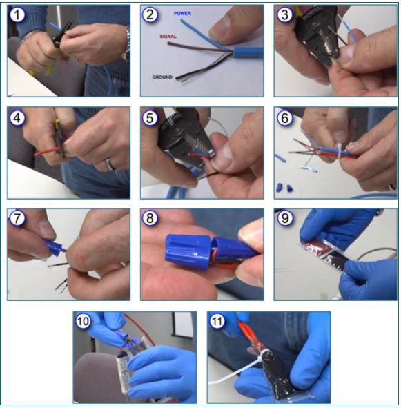
Assemble the Epoxy Seal Pack for Waterproof Electrical Connections
