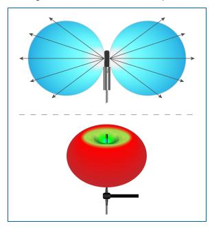
To have the best reception without signal loss, the antennas must be pointed in the same direction.
