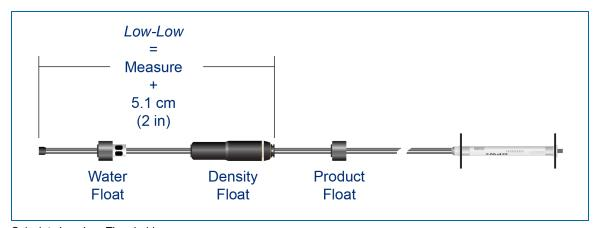
Calculate Low-Low Threshold Calculate Low-Low Threshold
