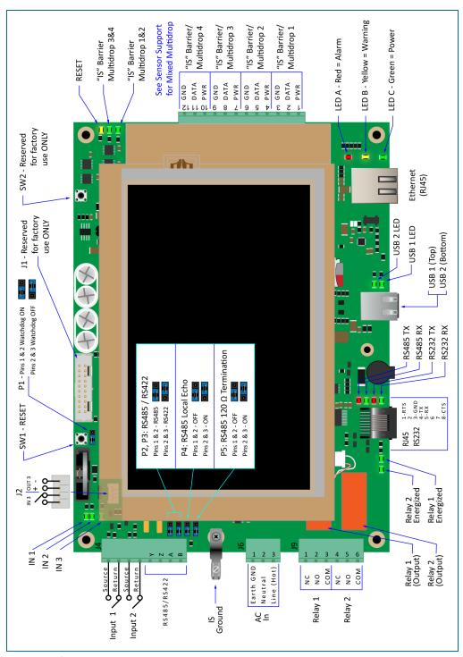
Main Board Connections, Jumpers and LEDs
