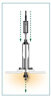
• Carefully install the assembled probe through the riser and flange into the tank.
