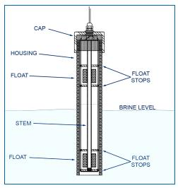
Cutaway View of Sensor Showing Internal Floats
