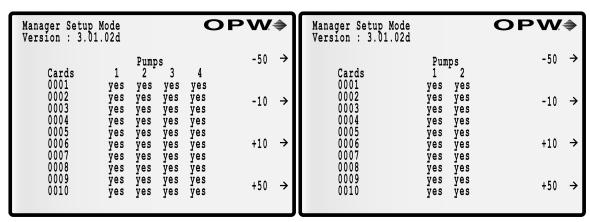
Allowed Pumps - 4 Pump Setup & 2 Pump Setup
