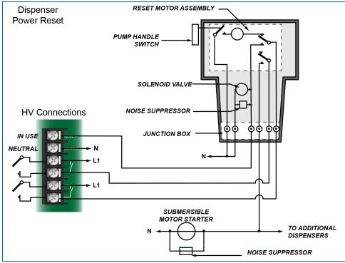
Typical Wiring for Dispenser with Power Reset
