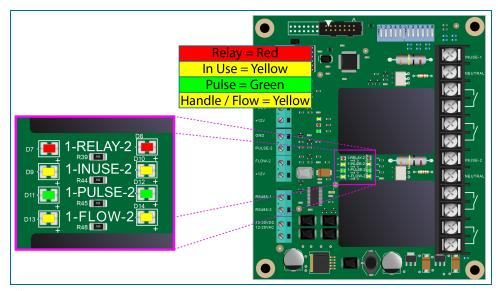
PCM Relay LEDs
