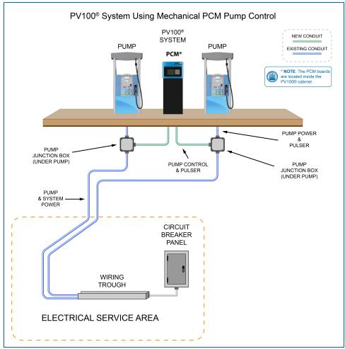
Typical Installation Overview with PCM Pump Control
