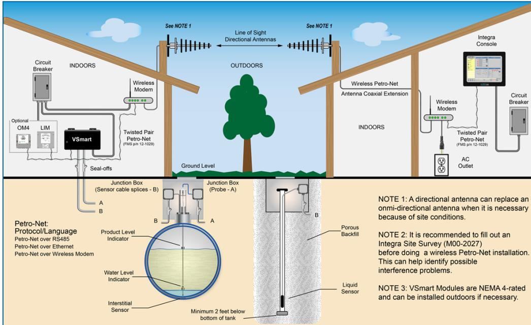
Figure 2-1 Wireless Petro-Net Installation with VSmart Indoors
