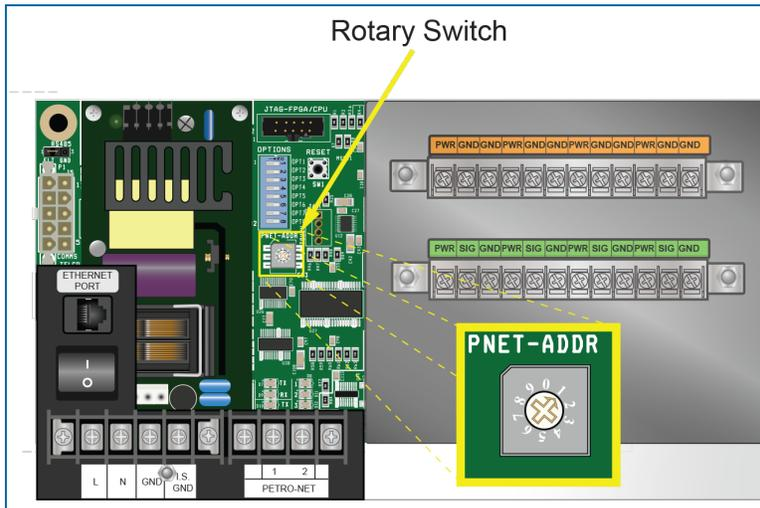
VSmart modules must be given an identification number to correctly communicate with the system through the Petro-Net protocol. This number must be different than all other VSmart modules in the system.
