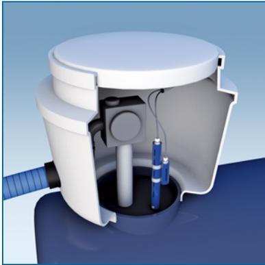
This sensor is made from the Hydrocarbon Liquid Sump Sensor (30-3219-12) with an Interstitial Level Sensor (30-3221-1A) attached. The primary function of this sensor is to sense liquid hydrocarbons and water in sumps, fuel dispenser pans and other locations where there is liquid that could indicate that a leak has occurred.
