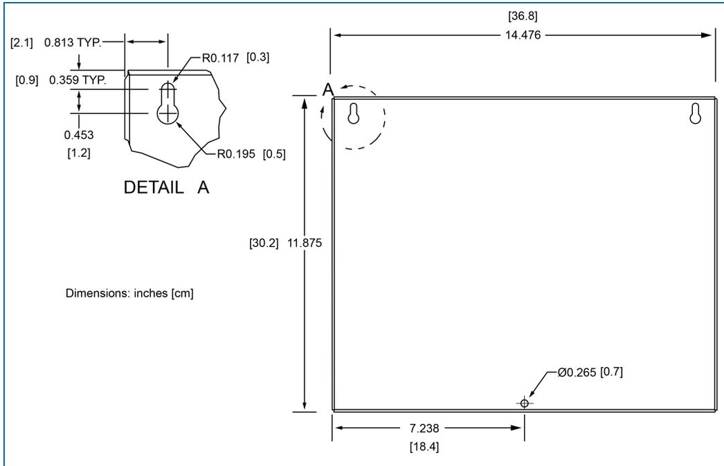
Figure 2-1 Rear Panel Install Hole Locations and Dimensions
