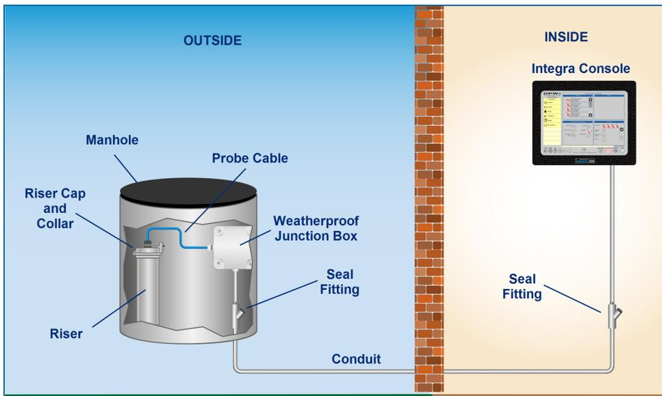
5. The cable must go through rigid steel conduit from the junction box directly to the I.S. barrier.
