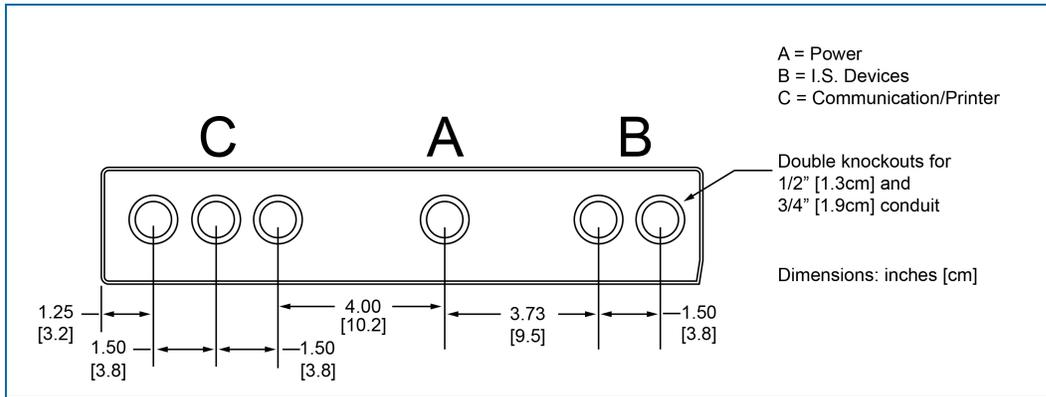
Figure 2-2 Console Conduit Knockout Locations
