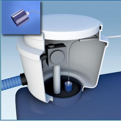
The primary function of the single-level sensor is to sense liquid in sumps, fuel dispenser pans and other locations where there is liquid that could indicate that a leak has occurred. A float inside the sensor moves up when the liquid level increases. The float switch will operate and cause an alarm condition in the controller. If there is a break in the cable it will cause an alarm condition in the system.
