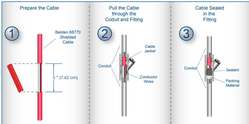
1. Prepare the Cable: Remove a sufficient length of the cable *jacket* so that the *conductor* wires can extend into the conduit seal fitting (approximately 3 inches [7.62 cm]).
