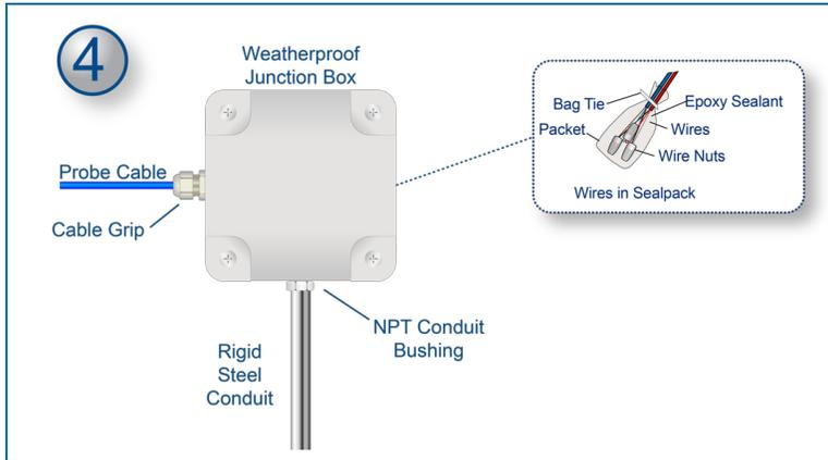
4. Tank-Probe or Smart Sensor wires that use a prepared Belden cable must go through NPT bushings into a weatherproof junction box. Bushings must be used in all junction boxes.
