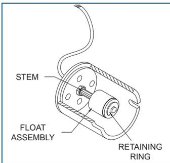
This sensor can also be used to monitor wet wells with normal liquid levels.
