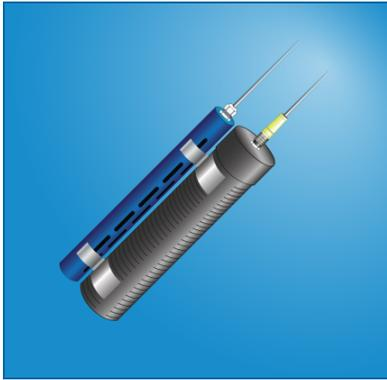
This sensor is made from the Hydrocarbon Liquid Sump Sensor (30-3219-12) with a Dual-Level Reservoir Sensor (30-3221-2) attached. The primary function of this sensor is to sense liquid hydrocarbons and water in sumps, fuel dispenser pans and other locations where there is liquid that could indicate that a leak has occurred.
