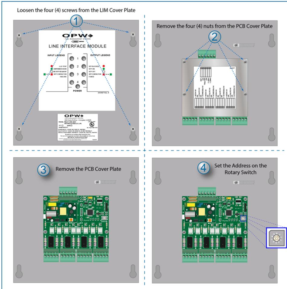
1. Loosen the four (4) screws that hold the LIM enclosure Cover Plate. It is not necessary to completely remove the screws. Move the plate so the screw heads align with the larger part of the screw hole slot. Remove the enclosure Cover Plate. Turn the plate around to get access to the PCB cover.
