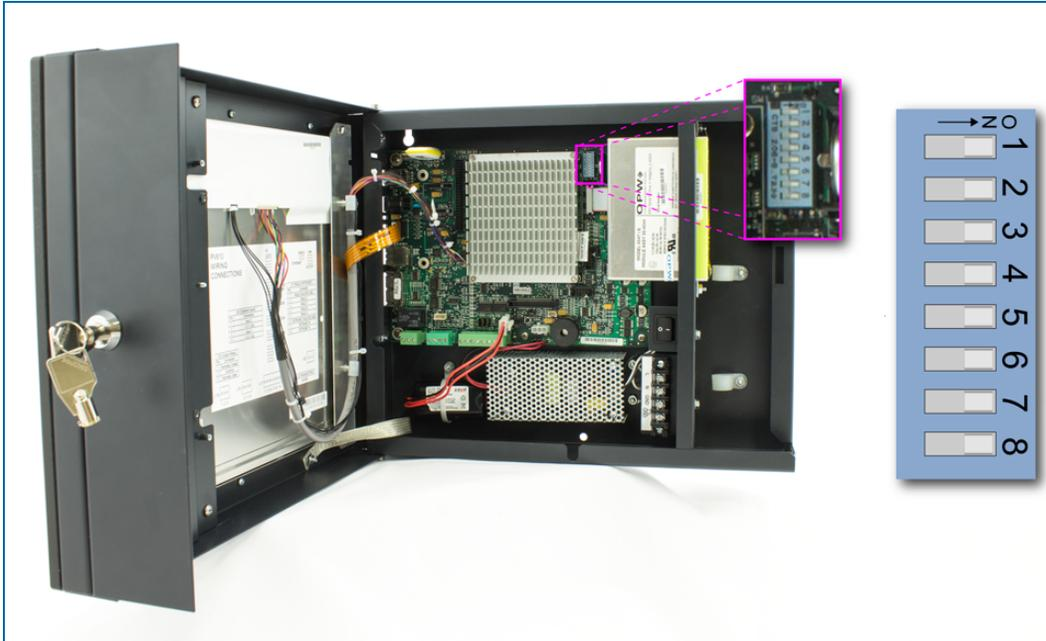
Figure 2-1 Main Board DIP-Switch Location and Configuration
