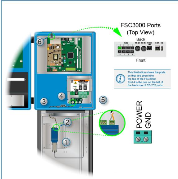
1. Attach the Isolated Converter (75-2036) to the mounting plate (51-0357) with two (2) of the 1-inch self-lock adhesive fasteners (50-2144).
