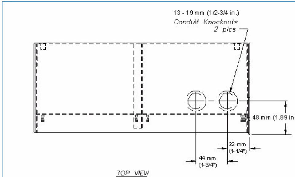
Figure 4-3 Controller Conduit Knockouts
