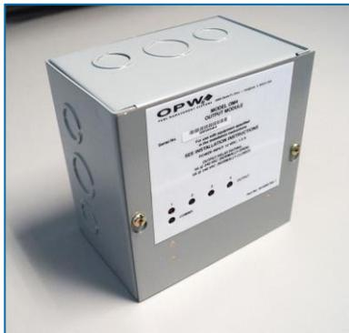
The **OM4** Output Module expands the tank-gauge console functions by allowing up to 2 (two) OM4 units each with 4 (four) relay positions for a total of 8 relays. The **OM4** communicates with the controller via Petro-Net™ and is powered by a 12 VAC wall pack source that is supplied with the unit. See the wiring instructions inside the **OM4** unit for the correct Petro-Net™ communications and power wiring connections.
