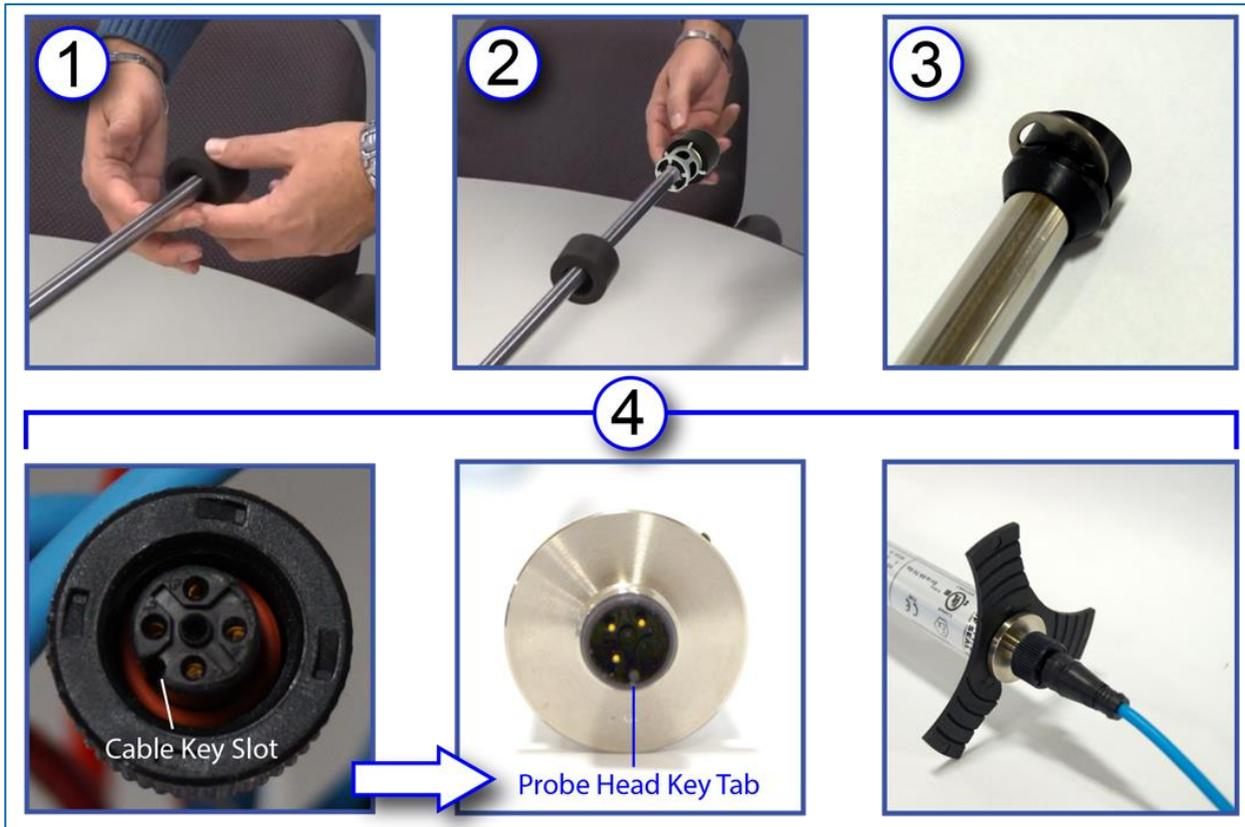
Figure 9-3 Probe Level Indicators and Cable Installation
