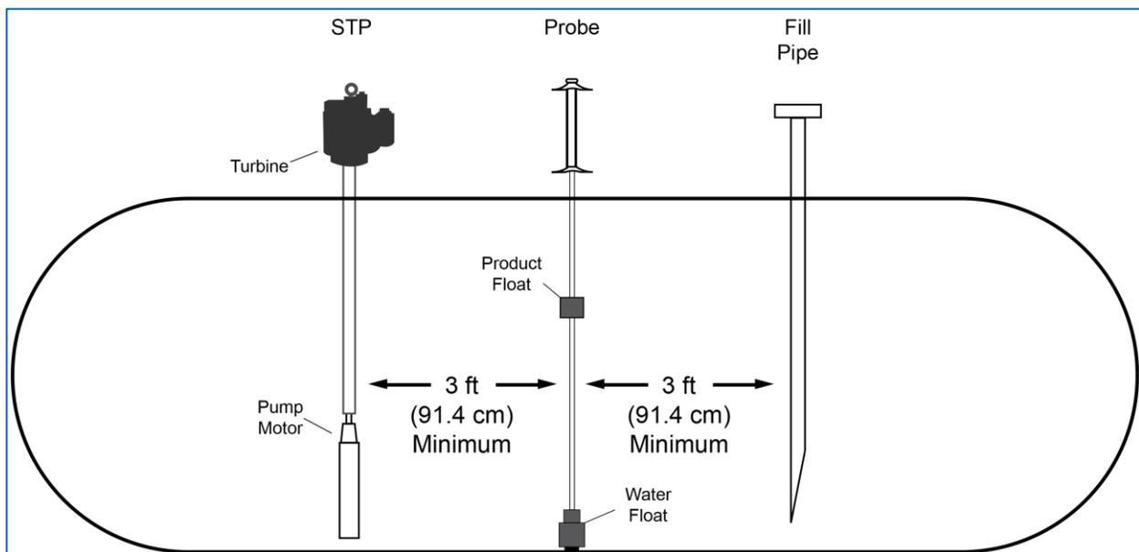
Figure 7-2 Probe Placement in Tank
