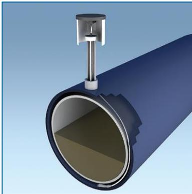
Figure 11-1 Interstitial Hydrocarbon Liquid/Water Sensor
