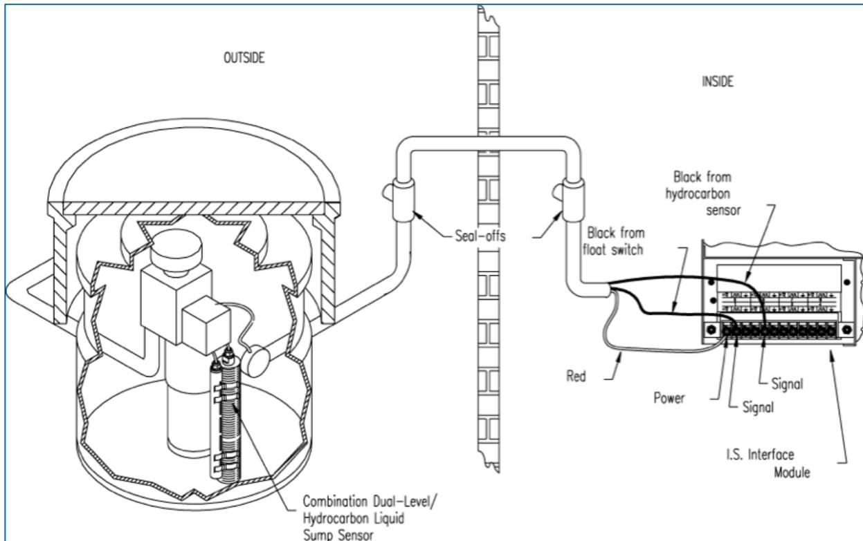
Figure 14-6 Combo Dual-Level & Hydrocarbon Liquid Sensor Installation
