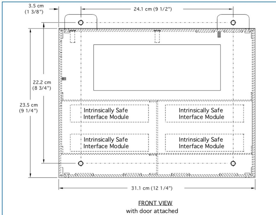
Figure 4-1 Mounting Footprint
