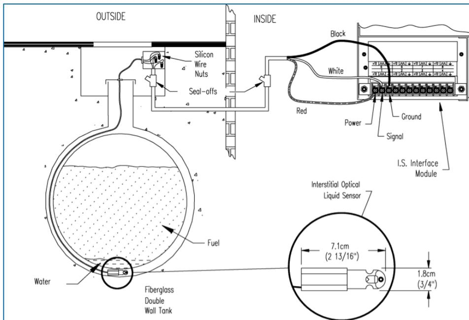
Figure 14-4 Interstitial Optical Liquid Sensor Installation
