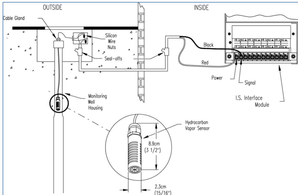
Figure 14-3 Hydrocarbon Vapor Sensor Installation
