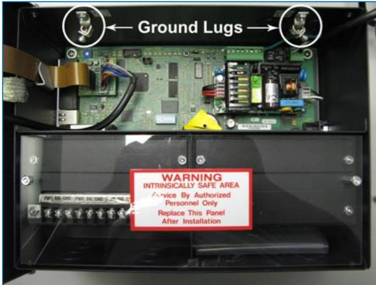
Figure 4-4 SiteSentinel iTouch Controller Ground Lugs
