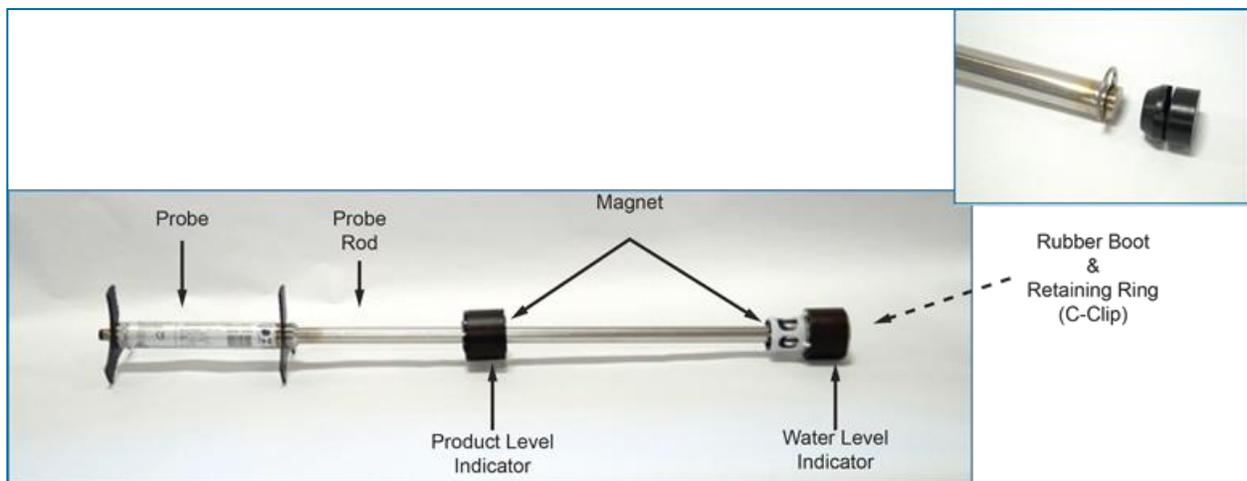
Figure 9-2 Probe Components
