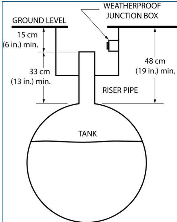
Figure 7-1 Underground Tank Manholes
