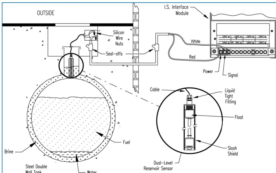
Figure 14-1 Dual-Level Sump Sensor Installation
