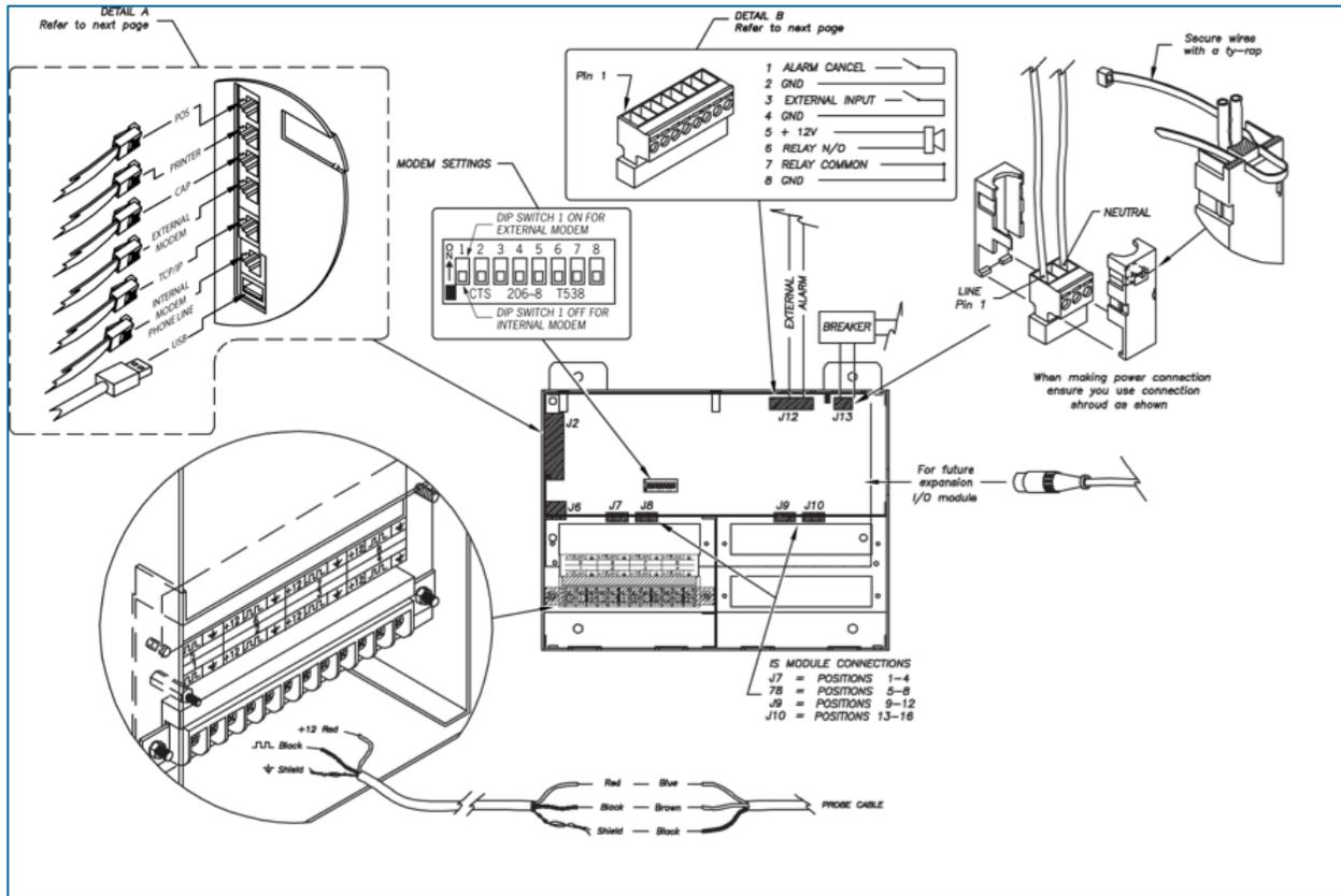
Figure 15-1 Connecting External Devices to the Controller
