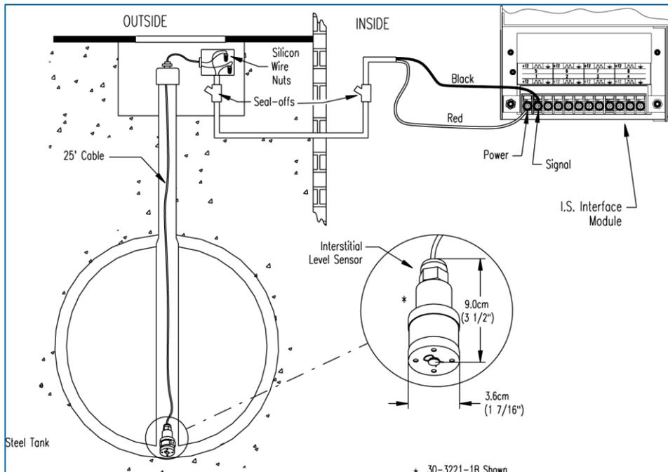
Figure 14-2 Interstitial Level Sensor Installation
