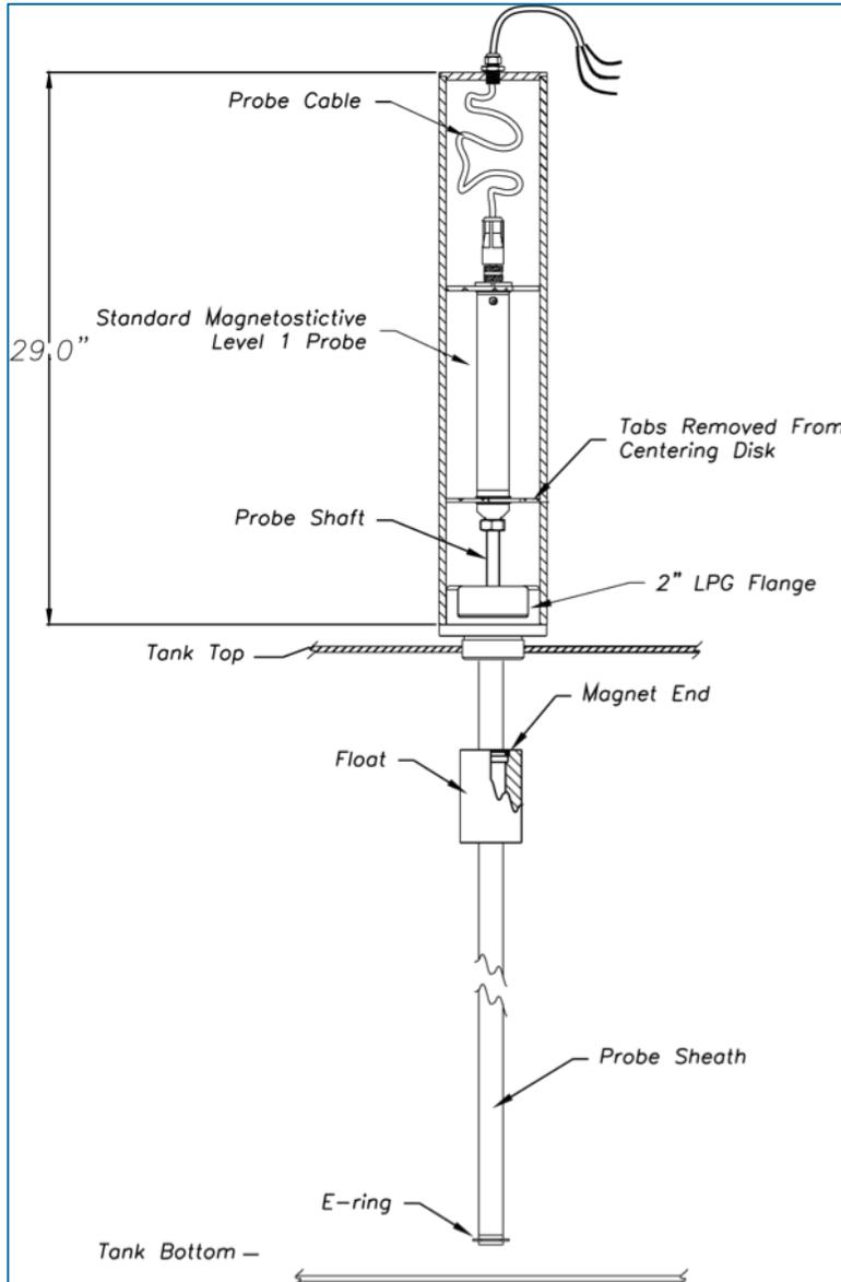
1. Slide the float onto the bottom of the probe fixture with the magnet pointing up.
