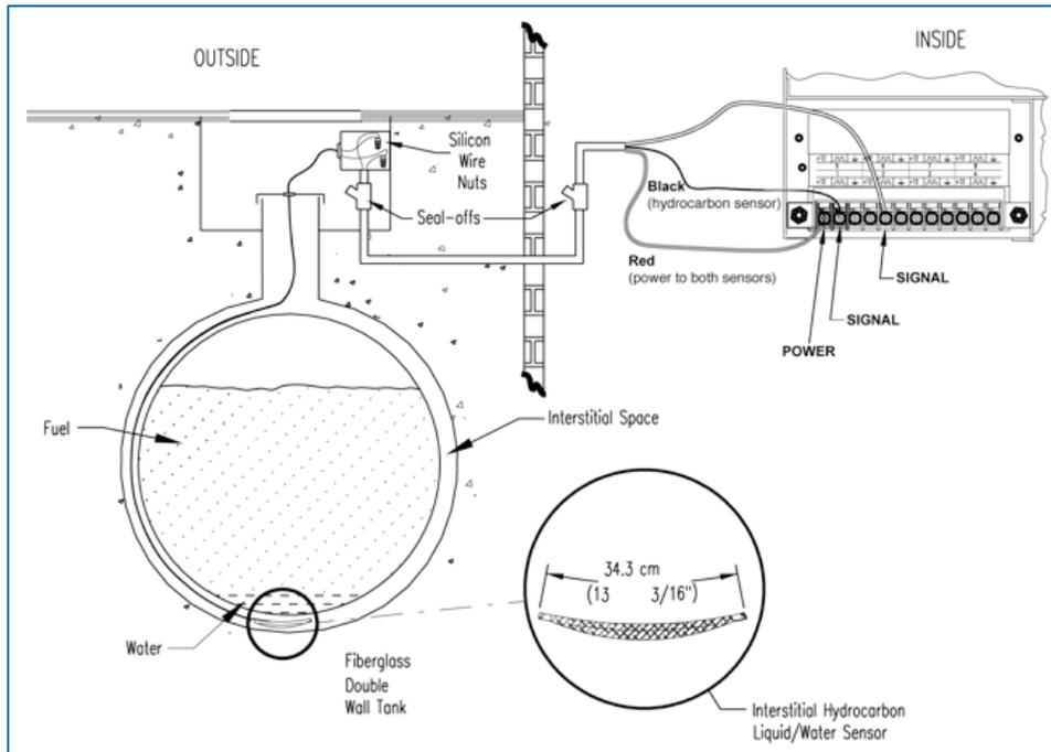
Figure 11-2 Interstitial Hydrocarbon Liquid/Water Sensor Installation
