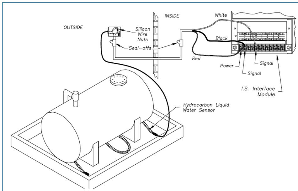
Figure 11-5 Hydrocarbon Liquid & Water Sensor Installation
