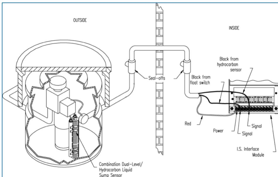
Figure 14-5 Combo Single-Level & Hydrocarbon Liquid Sensor Installation
