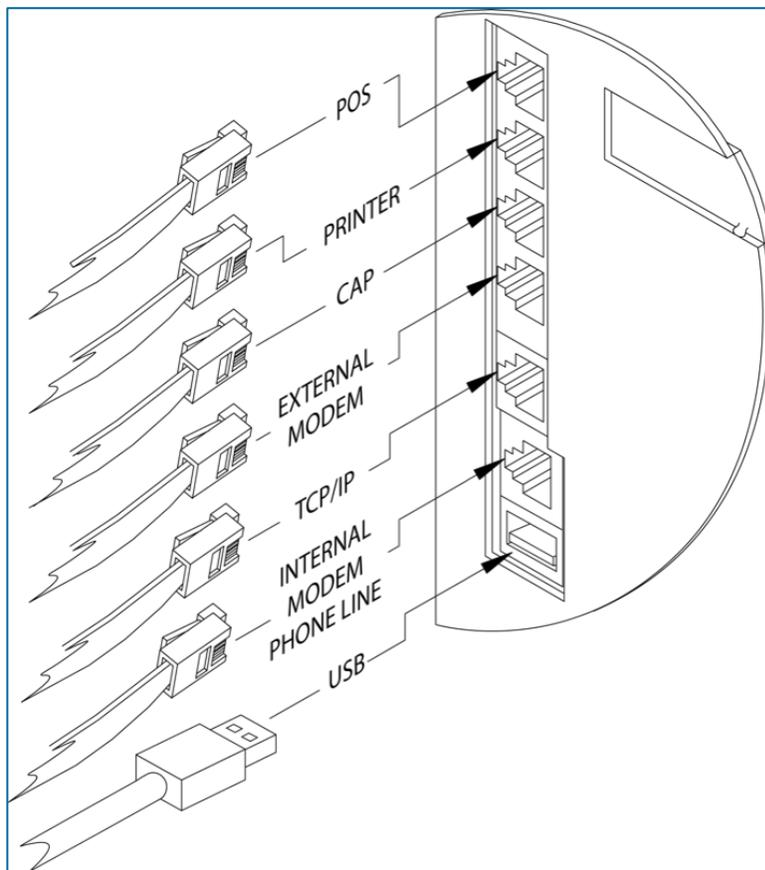
Figure 16-1 SiteSentinel iTouch RJ-45 Communication Ports
