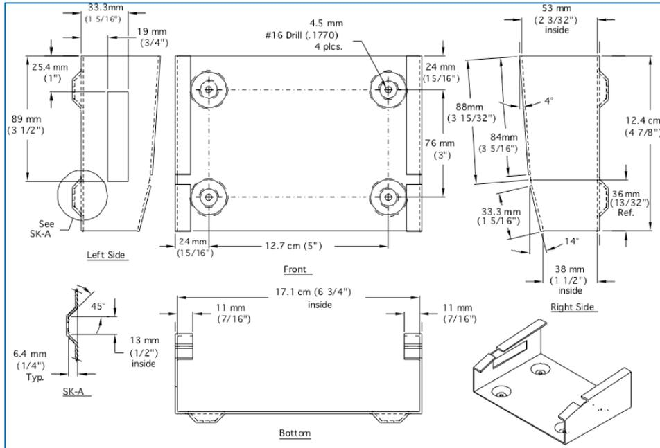
Figure 4-2 Printer Bracket Mounting Dimensions
