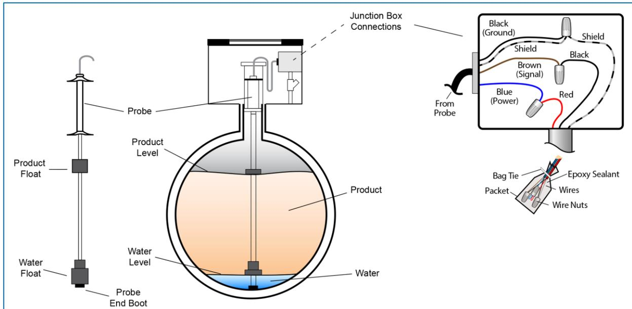
Figure 9-1 Probe Installation in Underground Tank
