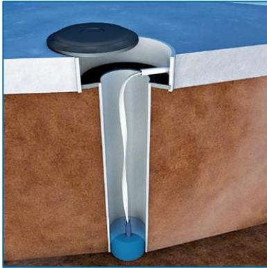
The hydrocarbon liquid/water sensor is used primarily in monitoring wells with fluctuating ground water tables or in containment areas of tanks, pumps and pipes.
