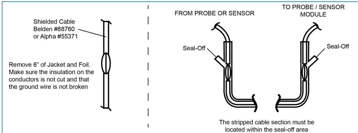
Figure 6-1 Probe Cable Seal-Offs
