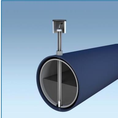
These two types of interstitial level sensors are used primarily in the interstitial area of a double walled tank. The sensors have a float switch that activates in the presence of a liquid. The **30-3221-1A** is constructed from chemical resistant, non-metallic material and the **30-3221-1B** is constructed from brass.
