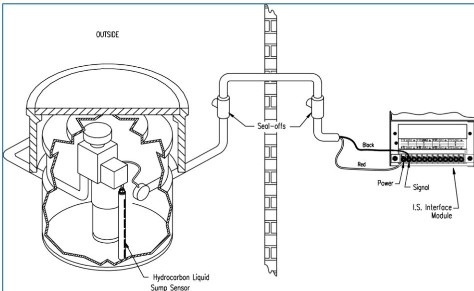
Figure 12-1 Hydrocarbon Liquid Sump Sensor Installation
