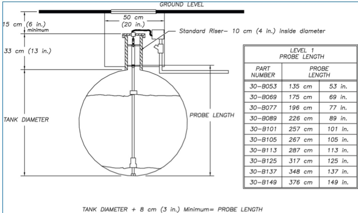
Figure 3-3 Probe in Tank Without Manhole
