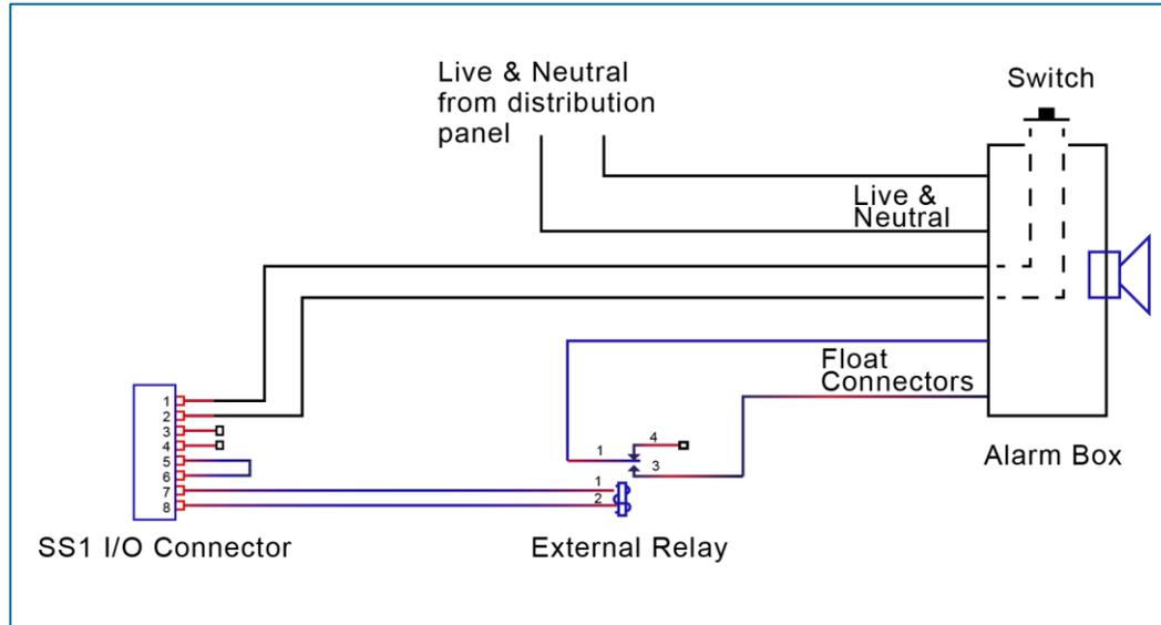
The Alarm Box will sound its horn and illuminate its light when the contacts close in the SiteSentinel iTouch Controller.
