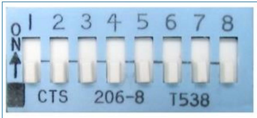
**NOTE:** DIP-Switch 1 is used for internal selection ONLY. Use the "On" position to select external modem; the "Off" is for internal modem. Once the dip-switch is changed, the SiteSentinel iTouch controller needs to be restarted. Dip-switch 3 is to select display type. Use "ON" for touch screen and "OFF" for keypad.
