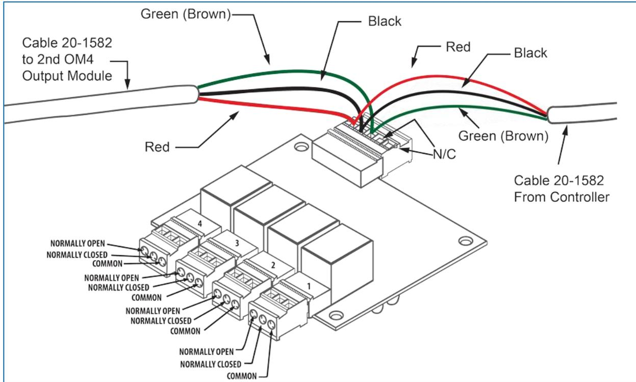
**NOTE:** When installing two (2) OM4 Output Module boxes, cut off the round DIN end of the remaining 20-1582 cable and use it to daisy-chain the POWER and SIGNAL terminals together. Route this cable through the conduit connecting the boxes installed earlier.
