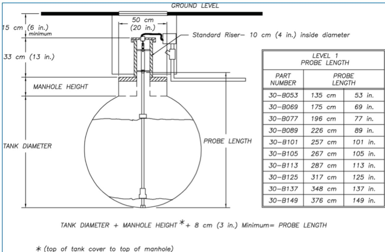
Figure 3-2 Probe in Manhole Equipped Tank
