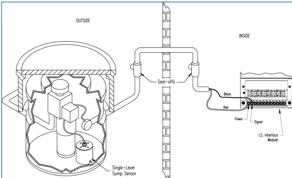
Figure 13-1 Single-Level Sump Sensor Installation
