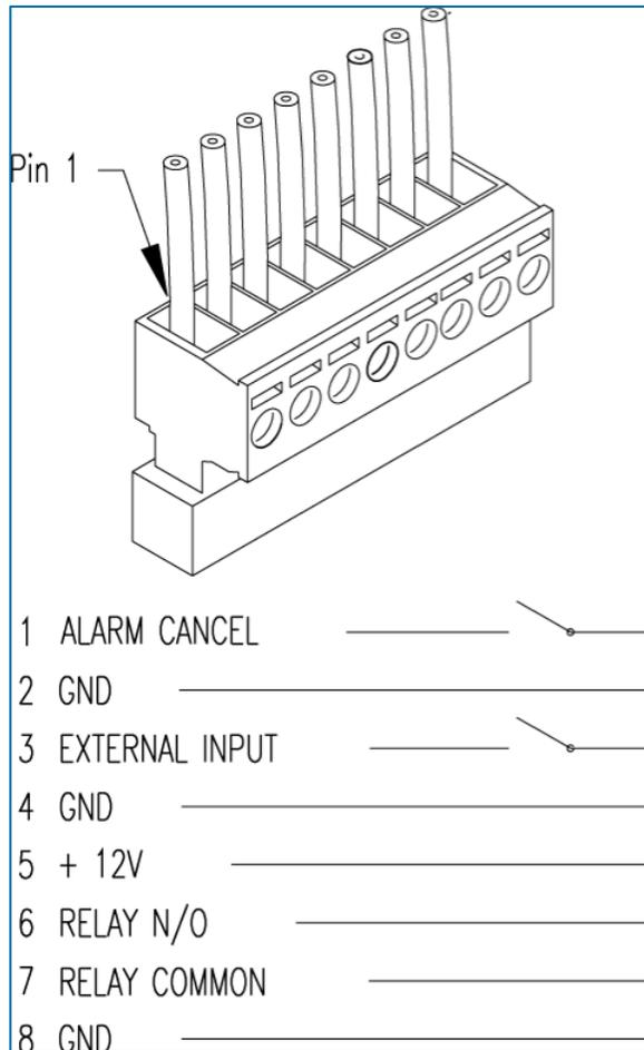
Figure 17-1 SiteSentinel iTouch Terminal Block Connections
