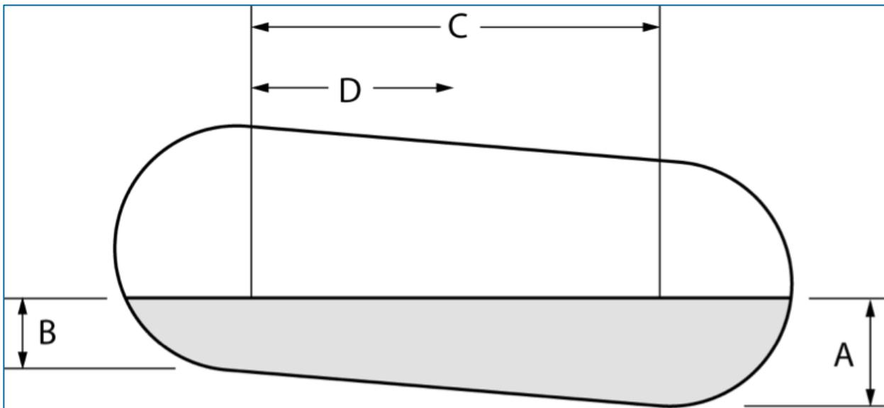
Figure 8-1 Calculating Tank Tilt
