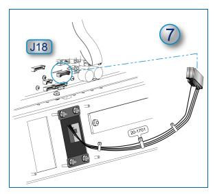
7. Connect the 9-pin connector of the Prox Reader Cable (20-1701) into the J18 connector (labeled "PROX READER") on the Main Board as shown.
