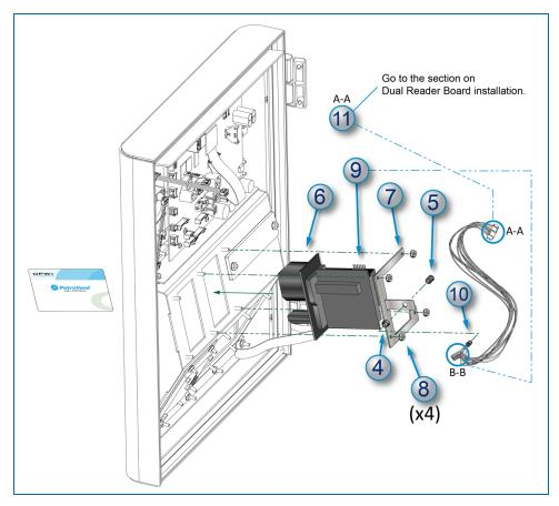
The LED Ring, Clip and Bracket are assembled at the factory for the upgrade kit. Reference steps 4-5 if it is necessary to assemble the parts in the field again.
