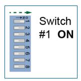
A DIP-Switch block in the top left corner of the controller board is used to open the Terminal Setup screen.
