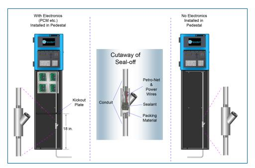
All conduits in the pedestal should terminate into a seal-off. The seal must be the first fitting where the conduit emerges from grade. Install 1/2" (1.3 cm) or 3/4" (1.9) rigid steel conduits, as applicable, to the area where the pedestal is to be located:
