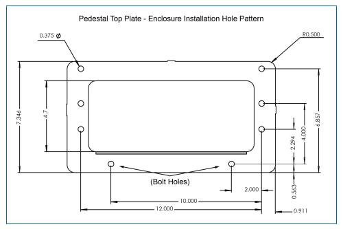
5. Use the provided hardware to attach the enclosure to the pedestal. Align the provided gasket with the mounting holes of the pedestal top plate. Carefully position the enclosure in place so that the open installation holes are aligned with the installation holes of the pedestal (see the illustration above). Put the four (4) bolts through the holes and tighten them using the provided washers and nuts.
