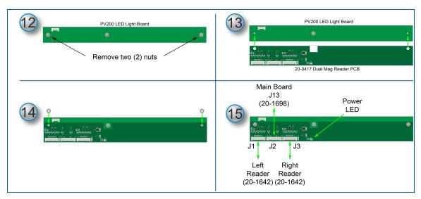
The 20-0417 Dual Mag Reader PCB will be installed on top of the PV200 LED Light Board. See the photo at the top of this instruction for the location of the LED board.
