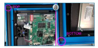
8. Remove the plastic strip from the back of one of the 17 inch pieces to expose the adhesive. With the adhesive face down, start at the top left corner and start the installation of this piece up against the 14 inch piece and against the edge of the door frame as shown. Carefully push down all the way along the gasket against the edge of the door frame to install the 17 inch piece. Make sure you do not stretch the gasket.
