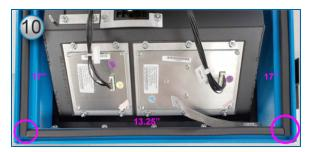
10. Remove the plastic strip from the back of the 13.25 inch piece to expose the adhesive. With the adhesive face down, start at the left and start the installation of this piece up against the 17 inch piece
