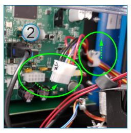
2. Disconnect the Power Supply harness from the Main Board (J16 Connector) and remove the harness wires from the cable clamp.
