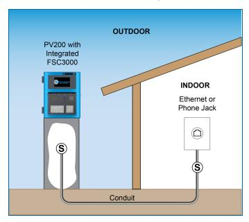
This conduit is required when you use a Terminal with an integrated FSC controller. This conduit will provide access for a phone line or Ethernet connection (300' [91.4 m] max.), or Serial Cable (50' [15.2 m] max.) to access the FSC.
