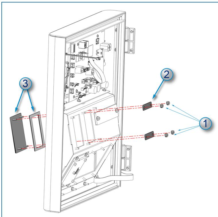
1. Remove the nuts from the blank-out plate screw posts for the applicable pocket slot where the card reader will be installed.
