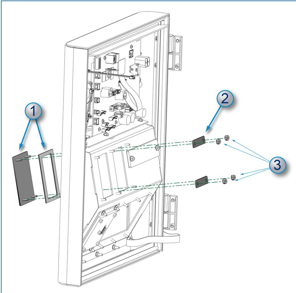
1. Put the posts of the Blank-out Plate (51-0451) through the gasket (50-2254) and the pocket slot from the outside as shown. Hold the Plate and Bracket in position.
