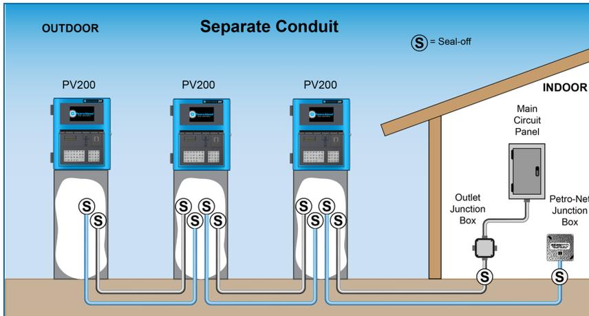
This conduit is required when you use RS-485 Communication wire that doesn't meet requirements to be installed in the Terminal Power Conduit, or you choose to have separate conduit. This conduit should run from where the Petro-Net junction box is mounted to each terminal. This conduit may be looped from terminal to terminal.
