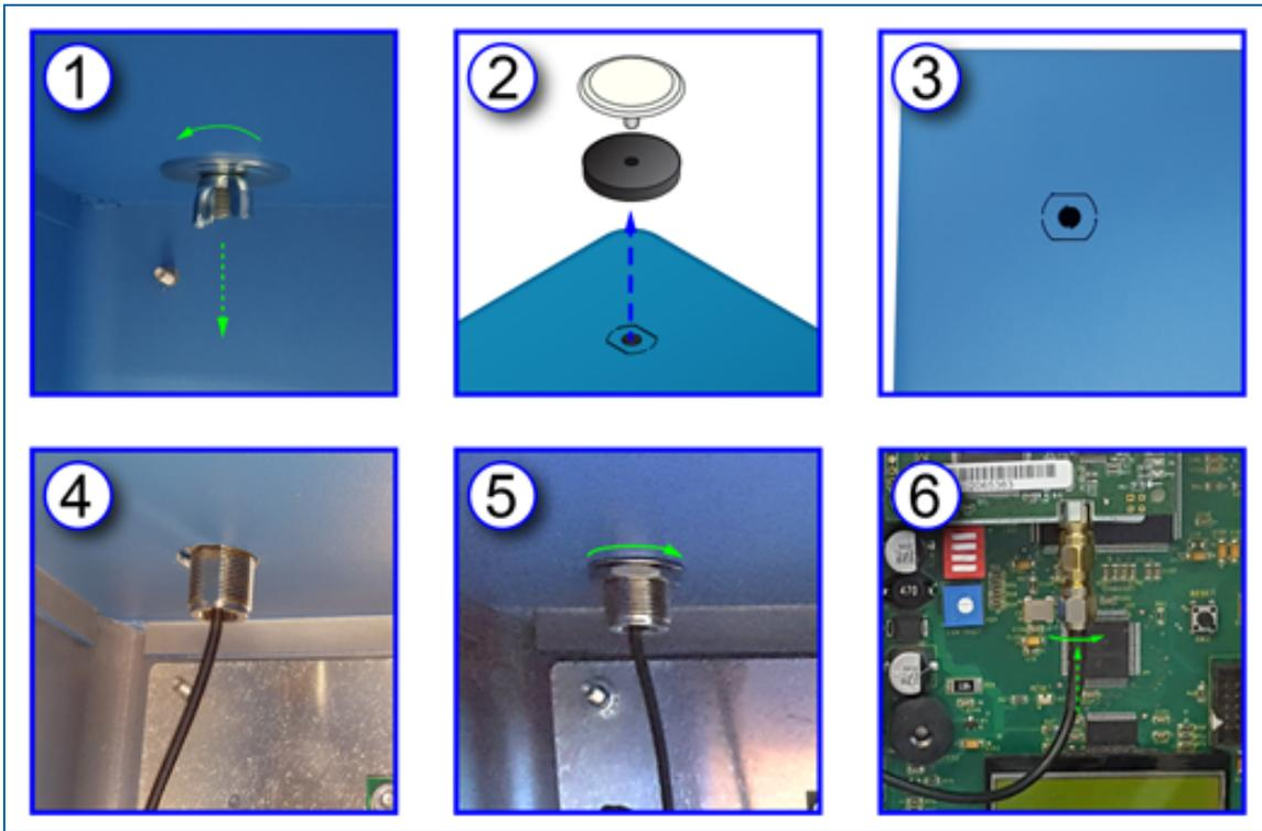
To install the 6" antenna to the enclosure for wireless operation:
