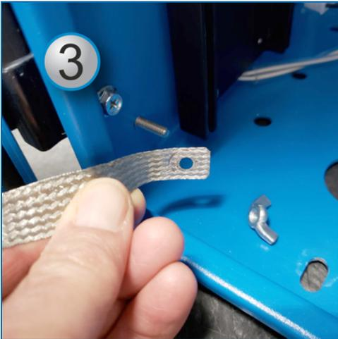
3. Remove the wing-nut that holds the Ground Strap to the Ground Post on the enclosure. Remove that end of the strap.
