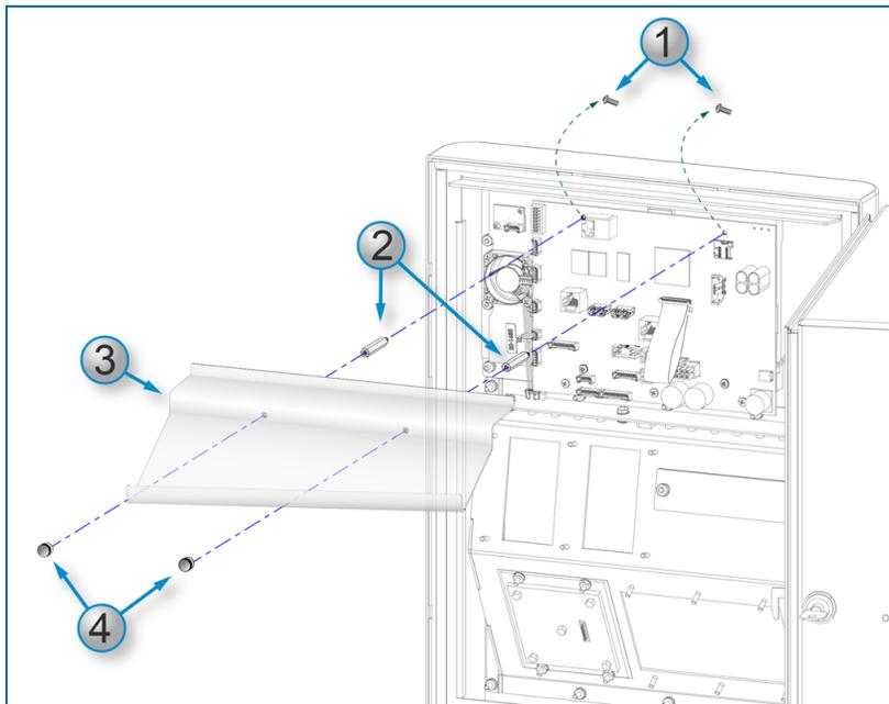
1. Use a Phillips screwdriver to remove the two (2) screws at the top of the Main Board as shown in the illustration.
