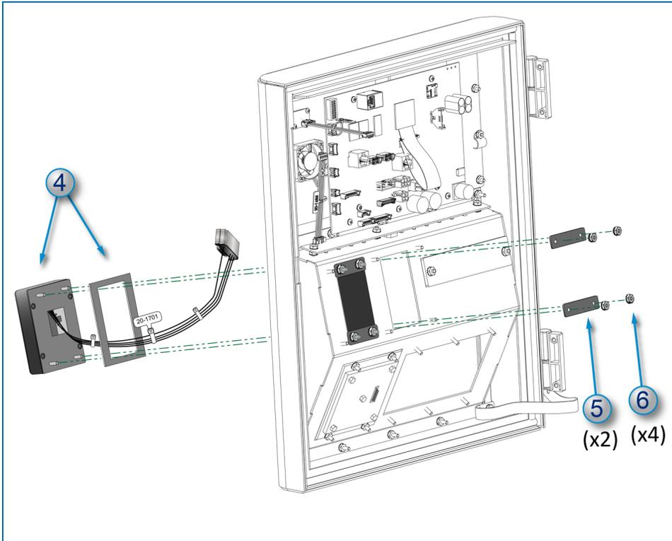
4. Put the Gasket (50-2254) around the pre-installed Cable (20-1701) and studs on the rear of the Prox Reader Assembly (20-4450). Put the Assembly with the Gasket through the open pocket slot until they are flush with the front panel of the pocket.
