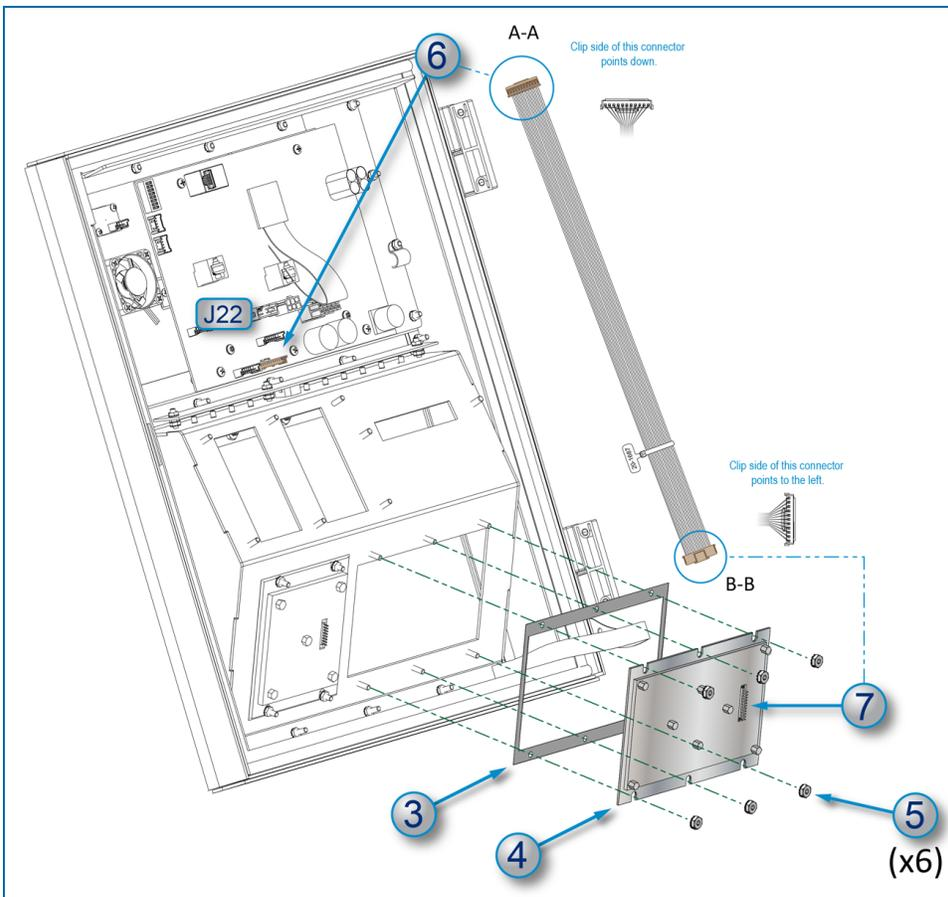
3. Put the Gasket (50-2253-A) over the six (6) pocket slot screw studs.
