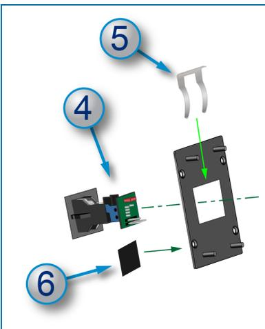
The ChipKey Sub-Assembly is assembled at the factory for the upgrade kit. If it is necessary to install a new ChipKey reader do steps 4-6 as shown below
