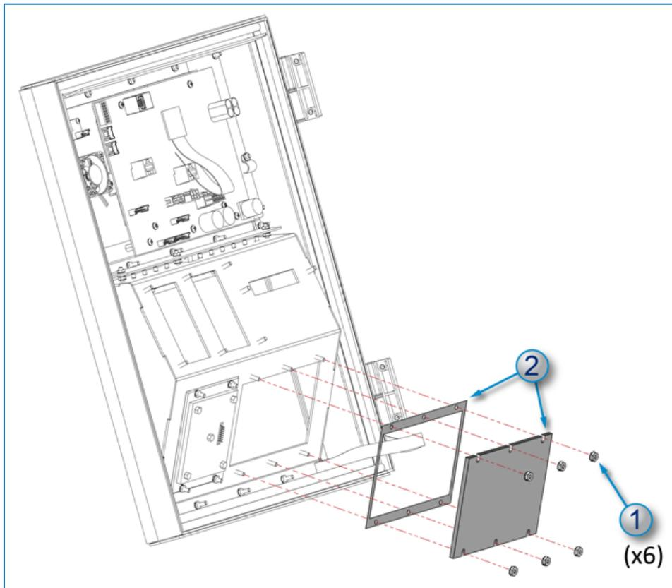
1. Remove the six (6) nuts from the pocket slot screw studs.
