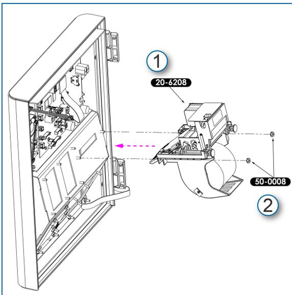
1. Put the printer unit (20-6208) onto the screw posts with the paper chute through the pocket slot.
