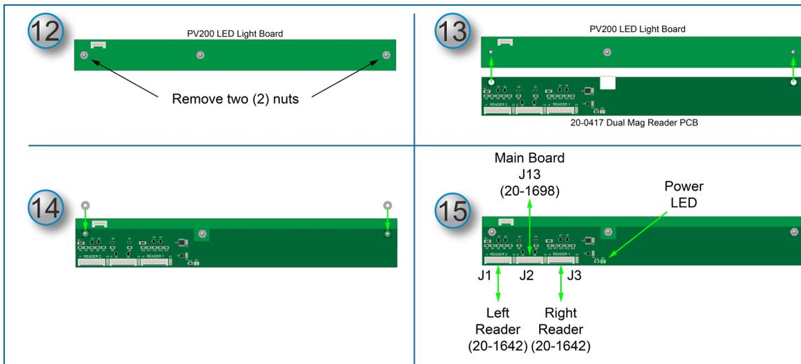
The 20-0417 Dual Mag Reader PCB will be installed on top of the PV200 LED Light Board. See the photo at the top of this instruction for the location of the LED board.
