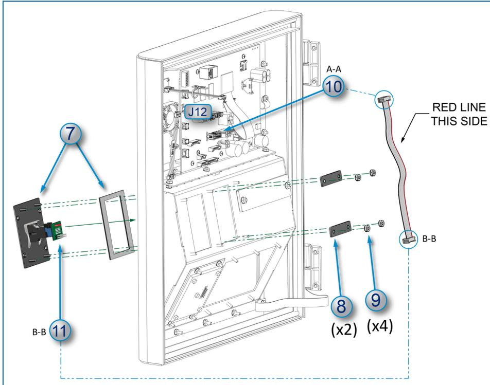
7. Put the Gasket (50-2254) around the ChipKey Plate studs. Put the Sub-assembly with the Gasket through the open pocket slot until they are flush with the front panel of the pocket.
