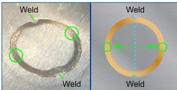
To remove the Knockout plugs in the bottom of the enclosure, hold a center-punch in the **green** circled areas shown in the illustrations above, and hit the punch with a hammer. The areas to hit are perpendicular to the
