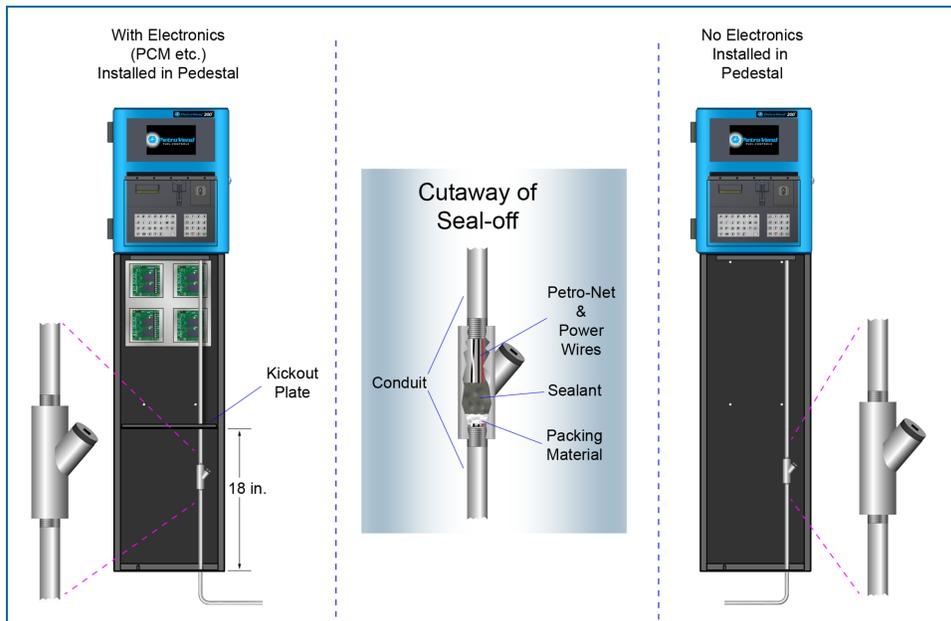
All conduits in the pedestal should terminate into a seal-off. The seal must be the first fitting where the conduit emerges from grade. Install 1/2" (1.3 cm) or 3/4" (1.9) rigid steel conduits, as applicable, to the area where the pedestal is to be located:
