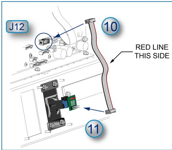
10. With the red line of the ribbon cable (20-1625) pointed to the right, connect the top cable connector into the J12 connector (labeled "CHIPKEY") on the Main Board as shown.
