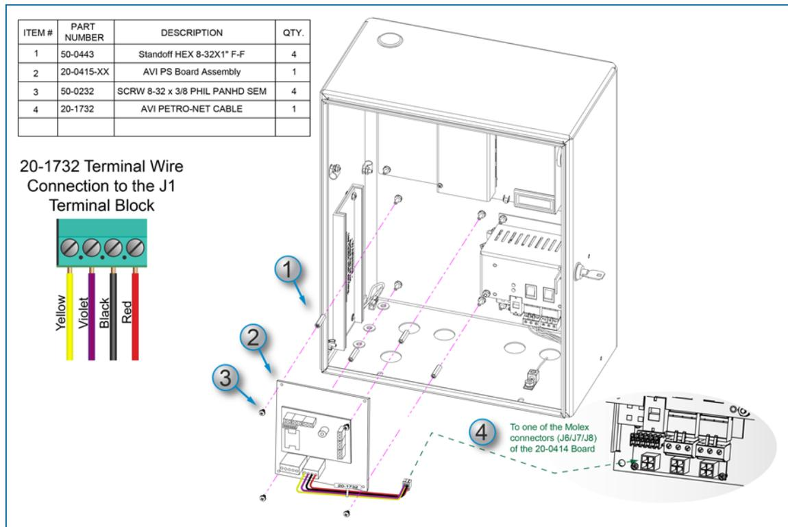
1. Remove the nuts from the studs on the back wall of the PV200 enclosure where the VIS Controller Assembly is to be installed.
