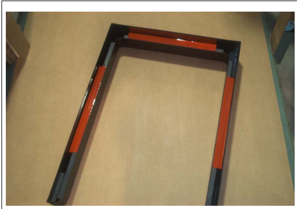
Figure 3. Remove Backing From 3M Tape
