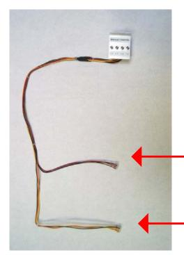
Connector with Black, Brown and Red wires connects to **top** PCM Master board
