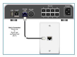
With the supplied RJ11 phone cord (FM12-3017), connect the modem connector on the rear panel of the FSC3000 to a working phone outlet.
