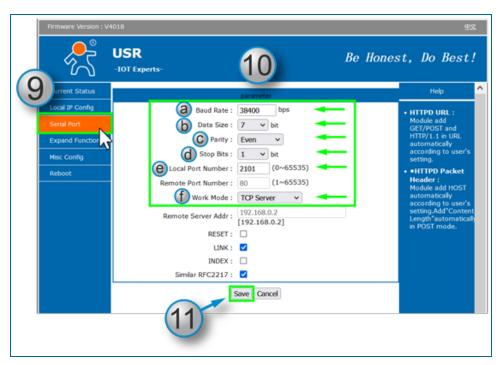
9. After you configure the necessary network settings, you can also configure the device's Serial port if necessary. Select the **Serial Port** tab in the left side menu.
