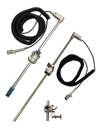
CIVACON Portable "Cane Probes" provide for portable overfill detection in cargo tank and rail tank car loading operations where a fixed sensor is not installed or is impractical to use, such as top loading of railcars. When properly used, our Portable "Cane Probe", in conjunction with and when connected to a CIVACON compatible Loading Rack Monitor, will help ensures that an impending overfill condition in the railcar or tank is properly detected.
