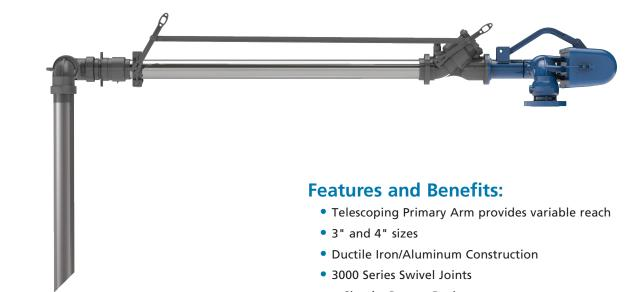
The slide sleeve type loading arm incorporates a slide-sleeve assembly that telescopes in and out to adjust for variations in the distance from the loading rack to the tank truck. It is used primarily in small bulk plants and terminals for top loading fuel oil or other petroleum products. This cost-effective loading arm is time-tested as a practical method of locating the drop tube accurately and easily.
