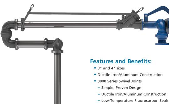
Primarily used to load tank trucks where the reaches will be less than 120" (3,048 mm). This versatile arm is designed specifically for top-loading installations where a variable operating range is required. The secondary arm rotates 360 degrees in the horizontal plane, providing a spotting allowance of up to twice its length.
