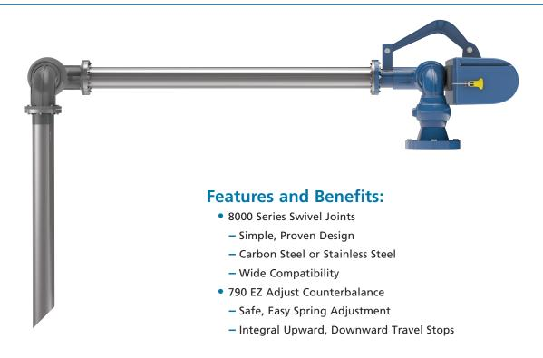
This simple arm incorporates only three swivel planes of rotation and is designed for use in top-loading installations where the vehicle is located at a fixed distance from the riser pipe. The two swivel planes at the inlet permit both up-and-down and side-to-side movement of the assembly, and the third swivel plane allows the drop pipe to remain vertical.
