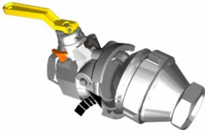
4. Once the jaw is engaged to the bottom of the nose, bring the body of the coupler in line with the adaptor by using the handle and push to engage the clamp to the top of the adaptor's nose
