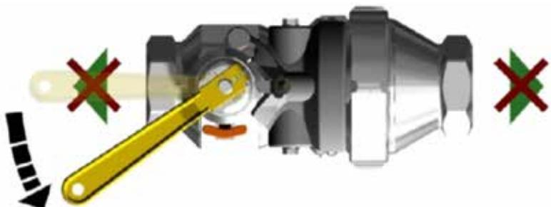
5. To lock the connected system in a closed position, view the connected system from the top, where the coupler is on the left and the adaptor is on the right, turn the handle counterclockwise until the lock engages
