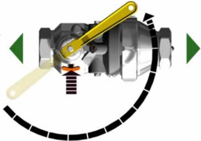
7. To close the system, press the safety release button on the coupler and rotate the handle clockwise until it locks
