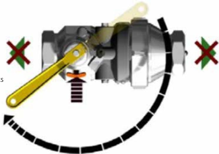
8. To disconnect the system, press the safety release button on the coupler and turn the handle clockwise so that it is parallel with the coupler. Press down on the clamp's tab (opposite side of safety release button) and push down on the handle to disengage the system
