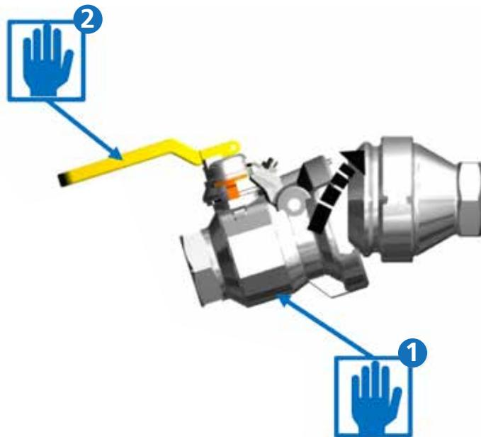
3. Bring the coupler towards the adaptor mating end at that upward angle, where the coupler's jaw would engage the bottom of the adaptor's nose first
