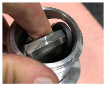
**14.** Place poppet axle (C4) into poppet (C3) hole to secure the poppet and guides (C15) in the body (C1)
