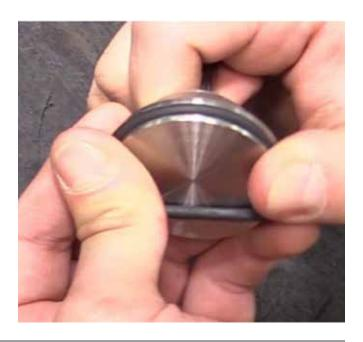
2. Place adaptor body (A1) face down on workbench, place the poppet (A2) face down into the body, and place the spring (A3) on top of the poppet
