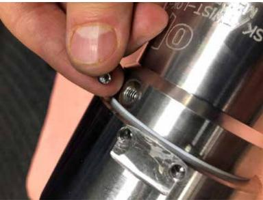
**19.** Position hand-wheel bracket (C19) on body followed by the hand wheel (C18) and thread bolts (C20) to secure wheel
