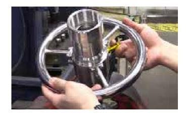
5. Rotate the coupler 120° clockwise to drive the poppet of the coupler forward, forcing the adaptor's poppet to retract and open the system for product to flow (note – the safety pin will pop into the adaptor groove once the coupler is rotated 120°)
