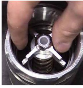
**4.** Compress the spring by pushing down on the bridge (A5); it is recommended to utilize a press to relieve the spring force
