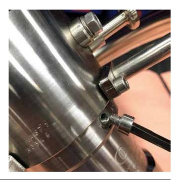
2. Pull swivel (2) from coupler body (C1), removing the swivel Teflon® washer (C8)
