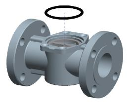
NOTE: EPDM seals are NOT compatible with petroleum-based lubricants. A silicone-based lubricant must be used with EPDM.
