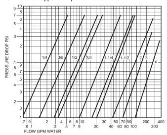
Minimum Flow\* Required to Turn Propeller
