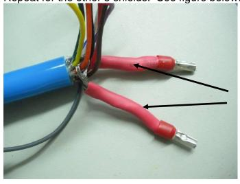
Heatshrink tubing and bootlace ferrules on the shields
