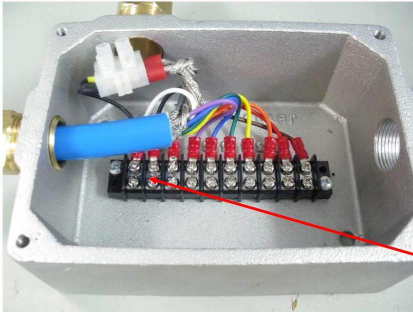
Shields connected to pin 10 in parallel with the white wire
