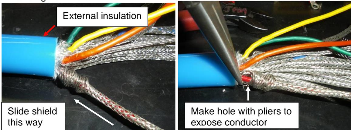
3. With a pair of long nose pliers separate the shielding at the base of the wire until the internal conductor is exposed. See figure above.
