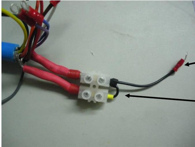
Fit ring terminal (Red M3) and connect to terminal 10 in the JB100 / JB103
