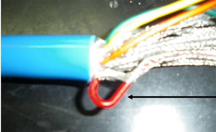
Pull cable through the hole in the shielding
