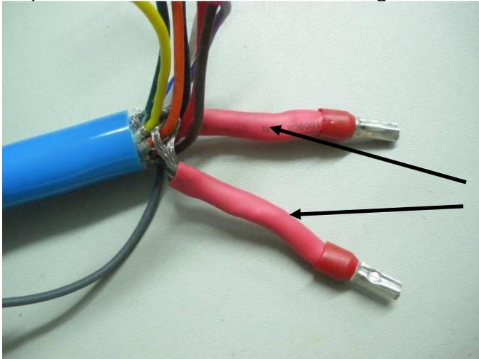
Heatshrink tubing and bootlace ferrules on the shields
