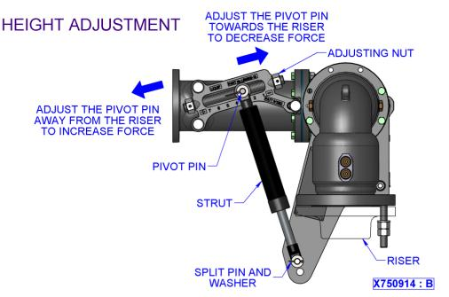
Figure 9: LBM800 Height Adjustment
