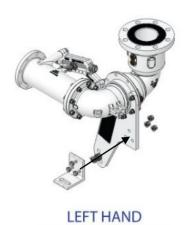
Figure 5: LBM800 assembly - Step 4
