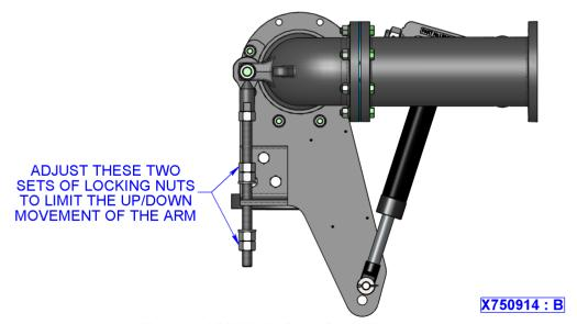
Figure 10: LBM800 Up-Down Stop Adjustment
