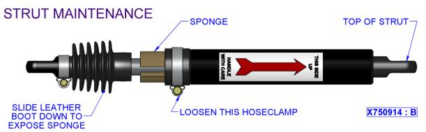
Figure 11: LBM800 - Strut Maintenance
