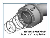
Step 7: Press static seal into swivel body outer groove, followed by placing purge seal inside recess created by tail and body. Set seal spacer ring inside purge seal, followed by main seal. Set SST smooth-bore ring inside main seal, then cap entire seal/spacer combination with sealing flange. Torque bolts to specified value.
