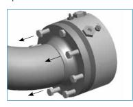
Step 6: Align flange with body and press surfaces together. Thread flange bolts with Nord-Lok™ washers into tail and torque to amount shown on chart. Nord-Lok™ washers come as an assembly bonded together from the factory. It is important that the correct orientation be preserved for proper function.
