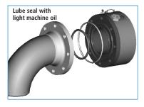
**Step 5:** Inspect and clean all machined surfaces. Press new static environmental and main seals into sealing grooves on swivel-module tail.
