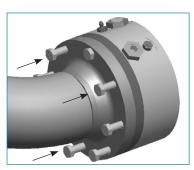
**Step 4:** With the rest of the loading arm still secured from movement, loosen the bolts on the other side of the swivel. Swivel module should fall away easily to expose environmental and O-ring seals. Secure product seal.
