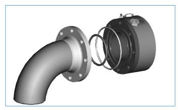
**Step 4:** Carefully remove dynamic environmental seal. Clean and inspect all machined surfaces and carefully press new environmental seal into groove. NOTE: Lube seal with light machine oil.
