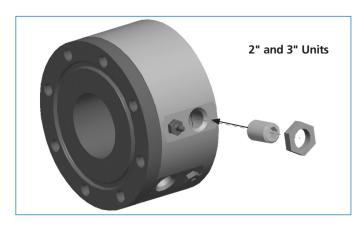
**Step 7a:** (2" and 3") With chamber completely full of bearings, rotate body/ tail until one bearing is directly in-line with the threaded ball-plug hole. Install the ball-bearing plug and tighten down until it is just snug on the ball bearing. Then install the jam nut. Loosen the ball-bearing plug by 1/2 to 3/4 of a turn and tighten jam nut.
