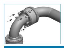
**Step 8:** Bolt sealing flange to body using bolts and Nord-Lok™ washers. Torque to amount shown on chart below.
