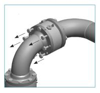
Step 2: Remove all split flange bolts on the side of the swivel attached to the free-moving end. With the bolts loosened, support this side of the loading arm along with any other parts attached to it that might move freely when the bolts are removed. Remove bolts, starting with lowest on flange, leaving top bolts for last. Be careful not to damage sealing flange module face and bolts.
