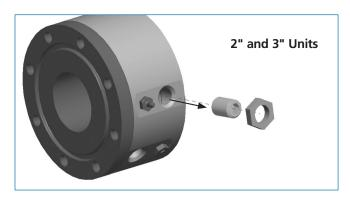
**Step 1:** Remove bearing plug bolts to access respective ball race.
