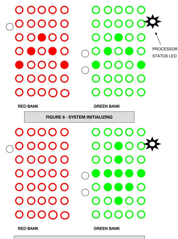
FIGURE 7 - GROUND IS VERIFIED (SEARCHING FOR OVERFILL)
