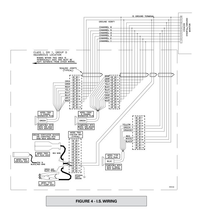
**Note:** Use optional earth ground when the monitor's earth ground is questionable in G/V plug or clamp source applications.
