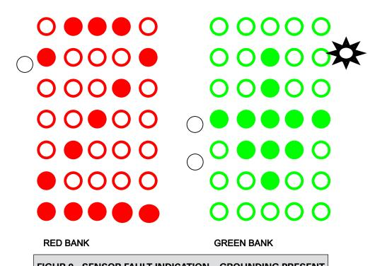
FIGUR 9 - SENSOR FAULT INDICATION – GROUNDING PRESENT
