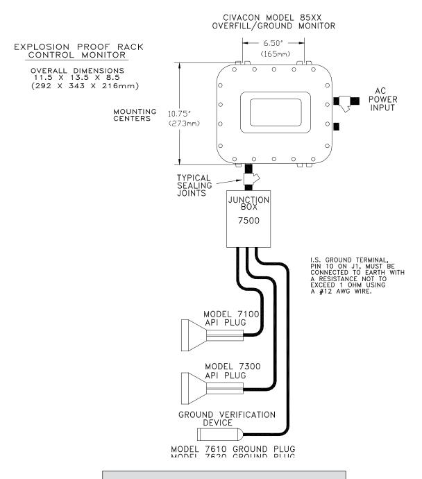
**FIGURE 1 - MECHANICAL INSTALLATION**
