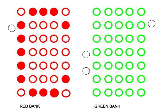
FIGURE 11 - COMMUNICATION FAULT - INTERNAL TO 85XX
